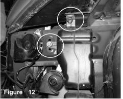
You will now need to remove the front bumper. Looking at the driver side corner, you'll notice the remaining two m6 bolts that will be removed from the air box resonator brackets. These bolts will need to be removed
