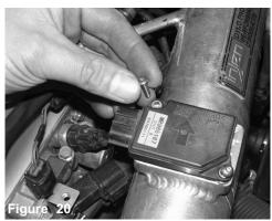
Place two M4 allen bolts onto the MAF sensor.
