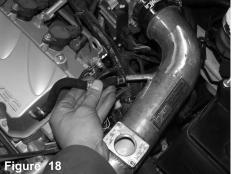
Connect the crank case breather line to the welded nipple on the intake pipe
