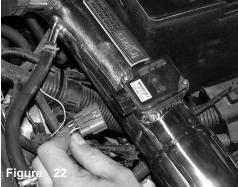
Re-connect the MAF sensor harness back onto the MAF sensor. Make sure you heard it snap in place.
