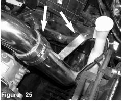
Connect the primary tube to the secondary tube while aligning the intake bracket to the vibra-mount.
