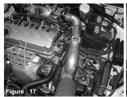
Position the primary pipe into the 2 7/8" straight hose located on the throttle body. Leave the clamp snug but loose to later adjust the pipe for best fitment
