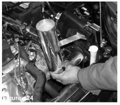
Lower the secondary intake into the engine compartment and into the opening leading into the bumper area.
