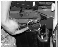
The m6 bolt is removed from the car frame. This bracket is attached to the plastic resonator box that will be removed. This is one of the three m6 bolts that will be removed.
