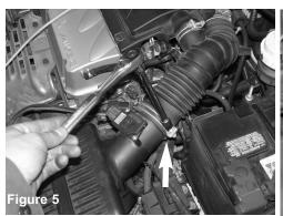
Loosen the clamp on the air duct attached to the air box assembly.
