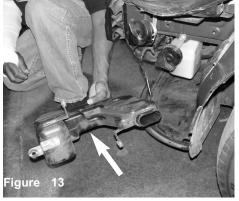
Once all three bolts have been removed, continue to pull the resonator box out.
