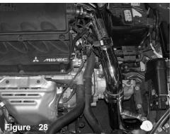
Use the m6 flange nut and fender washer to secure the intake bracket.
