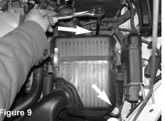
Use a 10mm socket, extension and rachet and loosen the two 10mm bolts on the air box assembly.
