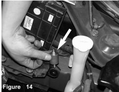
Screw the m6 vibra-mount into the front pre-threaded hole on the bracket used to mount the air box cleaner.
