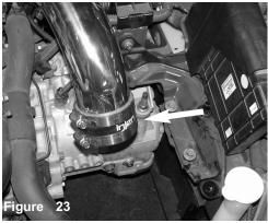
Press the 3" hose over the end of the primary intake. The 3" hose should not cover more than 1" of the edge of the intake. Use two power-bands and tighten the clamp on the intake side for now.
