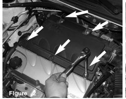
Use a 10mm Socket and rachet and remove the 5- 10mm Loosen the clamp on the intake air duct attached to bolts on the intake resonator located on top of the valve cover
