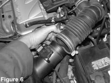
Detach the air duct from the air box assembly
