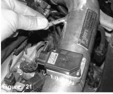
Use a 2.5mm allen wrench and secure the MAF sensor to the machined flange welded on the intake pipe
