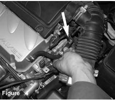
Detach the crank case breather line from the intake air duct
