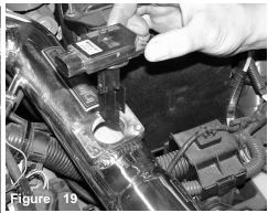
Locate the mass air flow sensor and insert it into the machined sensor adapter.
