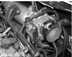
Place the 2 7/8" straight hose and two clamps on the throttle body
