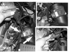
Flgure A: Use a torx screw driver to remove the two torx screw attached to the MAF sensor. Figure B: Unplug the MAF sensor harness. Figure C: Remove the MAF senor from the air box assembly
