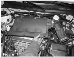
Remove the entire resonator box and air duct assembly out.
