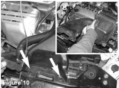
Figure A: Remove the two plastic screws on the air box scoop. Figure B: Remove the entire air box assembly
