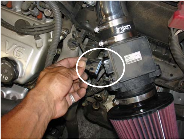
Reconnect the electrical mass air sensor harness prior to starting the engine.
