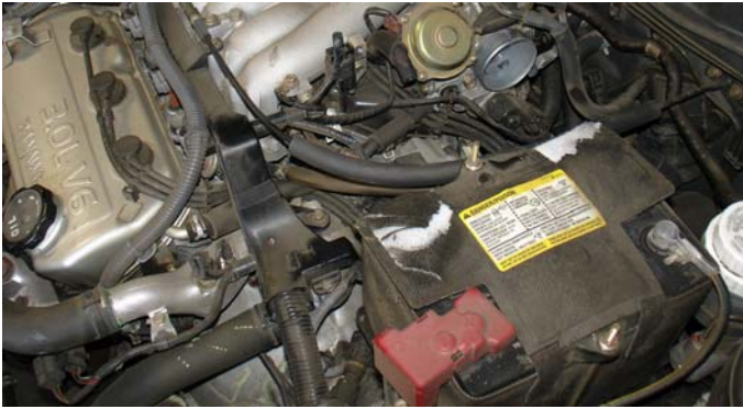
Engine compartment after the air intake box, ducts and air scoop have been removed.
