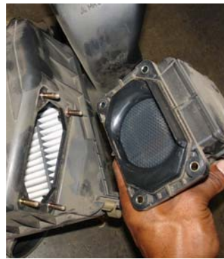
Remove the 4- 6mm nuts from the studs holding the MAFS to the air intake box as seen in the picture above.
