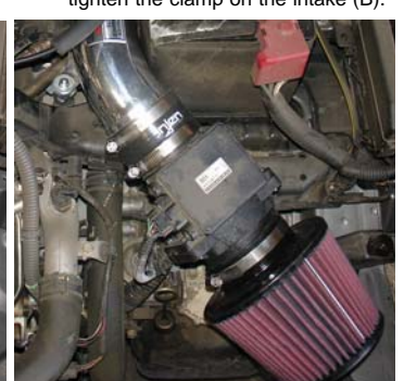
With the filter properly in place, align the intake for best possible fit.
