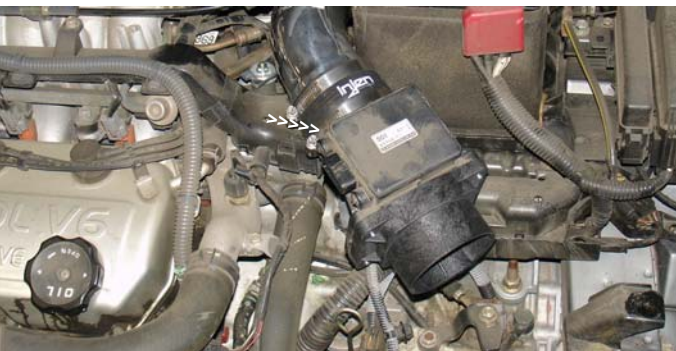
Take the assembled MAFS and press the outlet end into the 3 1/4" hose on the intake. Locate the MAFS for best fit and semi-tighten the large clamps used.
