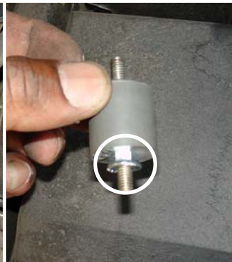
Take one of the 6mm flange nuts and place it on one end of the vibra-mount until it bottoms out.
