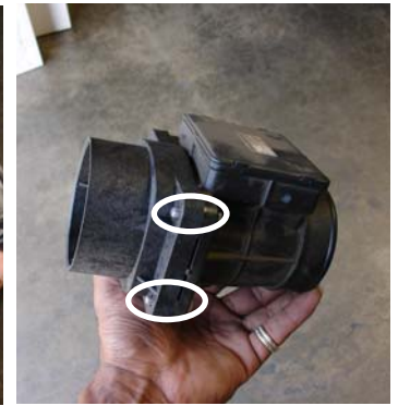
Take the flanged composite flange, butt it up to the flat surface of the MAFS. Use the 4- 6mm flange nuts to bolt the flange to the MAFS.
