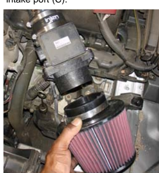
Press the 3 1/2" filter neck over the end of the composite flange.
