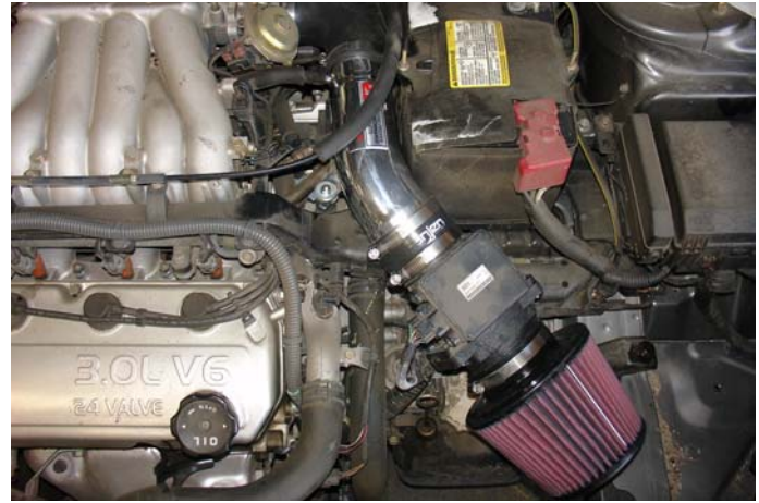
Align the entire intake for best possible fit. Check all lines, hose and fitment prior to tightening all nuts, bolts and clamps. Periodically, check the fitment of the intake and make sure it is not rubbing or hitting any moving parts.
