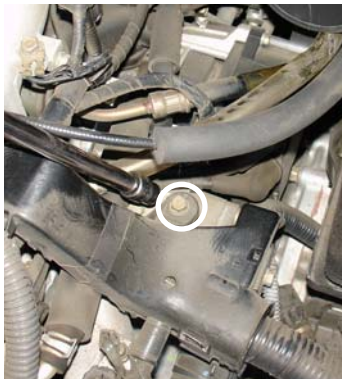
Remove the 6mm bolt seen in this picture. This is where the vibra-mount will be located.
