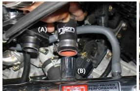
Take the 1 1/8" ID CCV hose, place two mini-clamps on each end of the CCV hose as shown above (A). Press the CCV hose over the large intake port as shown above.
