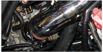
Press the intake throttle body side into the 2 3/4" hose. Align the intake bracket to the vibra-mount stud. Once the bracket has been aligned continue to semi-tighten the Power-band on the intake.
