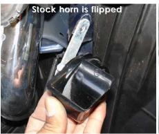
Turn the horn around so that it faces outward. Position the horn in place and screw the bolt back into the bumper frame.
