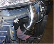
Locate the secondary intake and insert it into the bumper area via the engine compartment between the battery and front cross member
