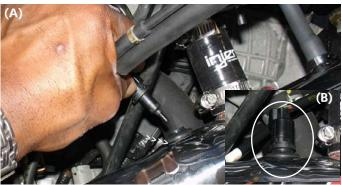
Press the air temperature sensor in to the 1525 sensor grommet (A). Insert the air temperature sensor into the grommet until it bottoms out (B).
