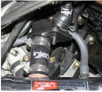
Once the CCV box has been correctly installed continue to tighten the mini-clamp.
