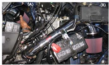
For short ram installation- Take the Injen filter and press it over the end of the intake (A). Once the filter has been properly installed continue to tighten the filter neck clamp (B).
