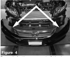
Remove the front bumper cover, using flat head screw driver, 6mm allen key, and phillips screwdriver. Carefully remove.
