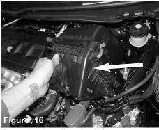
Remove the air box from the vehicle.
