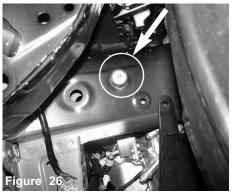
Locate the thredded insert on the vehicles frame below headlight, install and secure the vibra mount.
