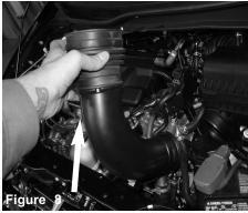
Now lift up and pull out the resonator tube.
