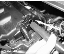
Install the provided 15mm hose to the engine.
