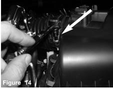
With 5.5mm socket and ratchet, loosen the clamp on the air box.
