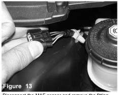
Disconnect the MAF sensor and remove the fitting from the air box.
