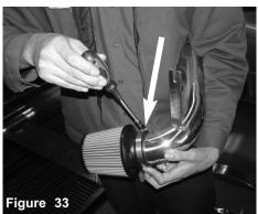
Install the air filter to the lower part of the intake assembly, secure and tighten using 8mm nut driver.
