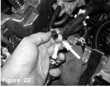
Connect the 2 lines together and secure using the factory clamp.
