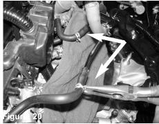
Loosen the clips on the hard line and slide back. This will be removed and secured with a 1/4" vinyl coupler. Note: Place a shop rag under neath and make sure vehicle is cold and not warm, there will be some coolant leaking.
