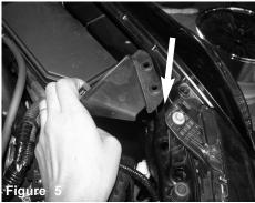
Disconnect the 2 push clips from the splash guard cover holding in the snorkel end of the air box located next to the battery.
