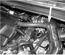
Secure the other end of the hose to the fitting on the injen Intake tube.
