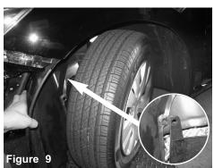
Turn the front tires all the way to the left. This will allow for easy removal of the resonator. Push back the splash guard also, remove any push clips holding the splash guard.
