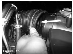
Pull back the intake tube from the air box.
