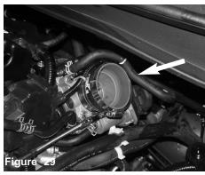
Install the step hose to the throttle body using clamps provided.
