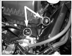
Loosen the 2 bolts that hold in the air box using 10mm socket and extension.
