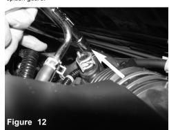
With pliers, loosen and pull back the crank case line from the intake tube.
