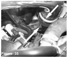
Now connect the 2 tubes and position for the best clearance. DO NOT TIGHTEN!
