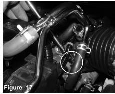
Loosen the the clamp on the throttle body using 5.5mm socket and extension.
