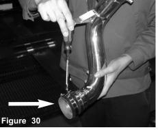
Install the 3" straight hose with clamps to the upper intercooler pipe, and secure on the intake tube only.
