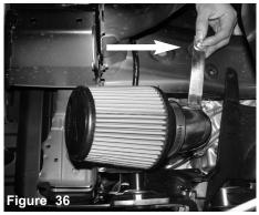
Now secure the lower part of the intake tube bracket using fender washer and nut.
