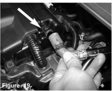
With pliers, loosen the clamp on the crank case line and pull back from engine. Next step will be to remove the coolant hardline which the Crank case line is attached to also.
