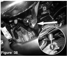
Now tighten both brackets using 10mm socket and ratchet.
