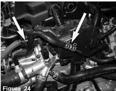
Now make sure the coolant line is secured and positioned like image above.
