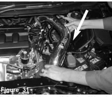
Intall the upper intake assembly into the vehicle and position to the throttle body and bracket to the vibra mount.
