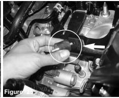
Now secure the m6 vibra mount to the factory thredded insert from the stock air box.
