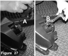
A) Loosen the 2 screws holding in the MAF sensor.
