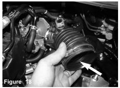
Pull any lines away from the intake tube and remove the intake tube from the vehicle
