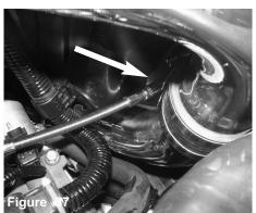
Position for the best fit and make sure there is clearance and nothing is touching or rubbing. Tighten all clamps using 8mm nut driver.
