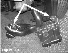
Carefully remove the resonator from the vehicle. Loosen the two 10mm bolts holding in the resonator. Note: This will require some force when removing from the vehicle, very tight fit.
