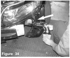
Now install the lower part of the intake assembly into the vehicle from the bottom, and position to the upper intake assembly. *Place provided vinyl trim to the frame to prevent contact of intake tube and frame.*
