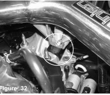
Position the intake tube for best fit and secure the bracket using provided fender washer and nut.
