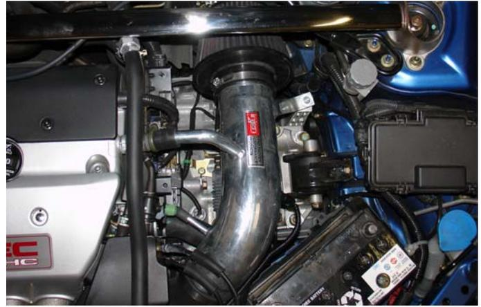
Once all air temperature sensors, vacuum ports and clamps have been located in place, continue to adjust the entire intake for best possible fit. Make sure that there is plenty of clearance through out the length of the intake prior to fastening all nuts, bolts and clamps.
