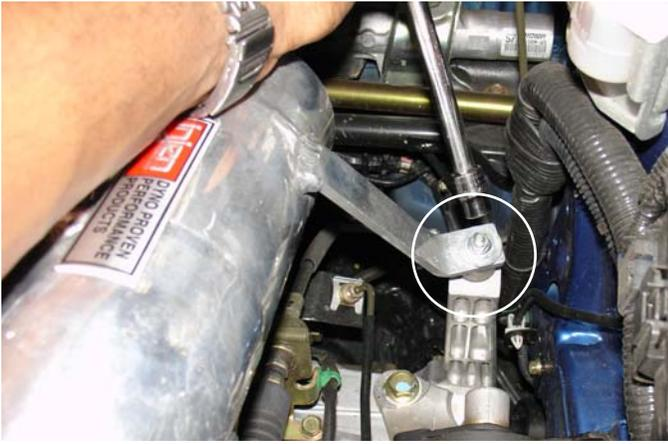
Once the vacuum port, air temperature sensor and breather line has been adjusted in the proper position continue to align the intake for the best possible fit. Take the flange nut and fender washer and fasten the intake bracket to the vibra-mount stud.
