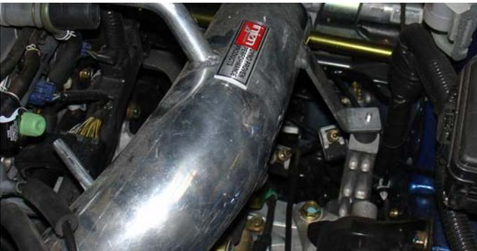
Align the MR Tech intake bracket to the vibra-mount stud then continue to line up all the other ports.
