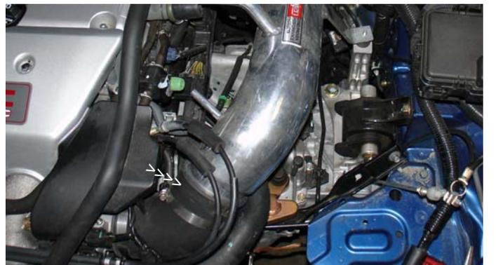
Once assembled, press the opposite end of the MR Tech intake into the three inch opening of the molded elbow.
