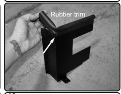
**19.** Install the provided rubber trim, to the top of the heatshield. Notch corner with pliers or cutters for easy install.
