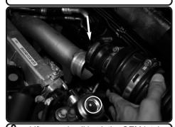
**8.** Lift up and pull back the OEM intake tube from the turbo housing.
