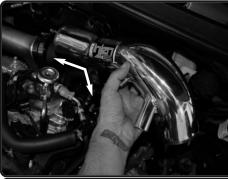
**15.** Now install the intake tube into the vehicle. Position the bracket on the tube to the vibramount. And the tube to the step hose.
