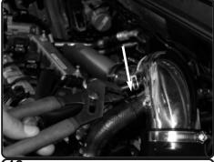
**18.** Connect the BOV line to the intake tube fitting and secure.
