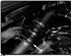
**5.** Loosen the clamp on the turbo housing using 10mm socket or wrench.
