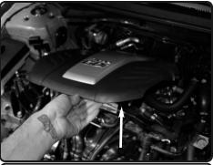
**3.** Lift up and remove the engine cover from the vehicle.
