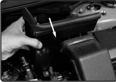
**21.** Now install the heatshield to the vehicle, install and place factory scoop through hole cut out.
