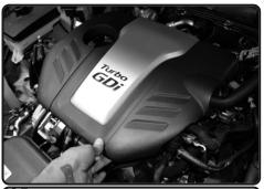
**25.** Re-install the engine cover and secure.
