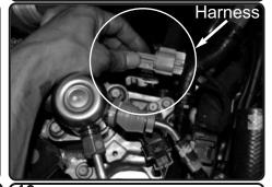
**10.** Locate this harness on engine. Pull back the plastic fitting away from the black metal bracket.
