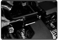
**22.** Now secure and tighten the bracket on heat shield using 10mm socket with extension.
