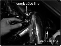
17. Connect the crankcase line and the vacuum line to the intake tube.
