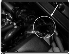
**7.** With pliers, pull back the vacuum line away from OEM intake tube.
