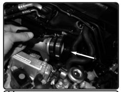
**14.** Now install the step hose with clamps provided to the turbo housing. Tighten the clamp on turbo housing only.
