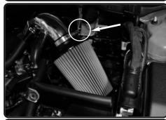
**23.** Install the air filter to the intake tube and tighten using 8mm nut driver.
