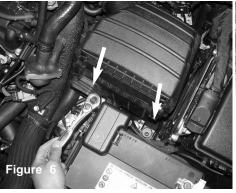
Use a 10mm socket/rachet and remove the two M6 bolts in front of the air box assembly
