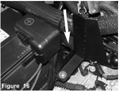
Photo showning air diverter attached behind battery Arrow indicate where the slot where the factory air box inlet duct will be re-installed from figure 5
