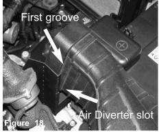
Top view of the inlet duct placed into the slot of the air diverter. Make sure you line up the first groove with the slot on the air diverter.
