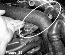
Lift the factory upper intercooler pipe up and slide the Injen intake pipe bracket underneath the upper intercooler pipe bracket
