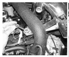
Place the supplied longer M8x40 bolt into the hole of the factory upper intercooler pipe bracket
