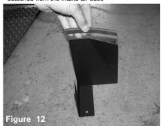
Place the supplied vinyl trim onto the top of the Injen Air Diverter
