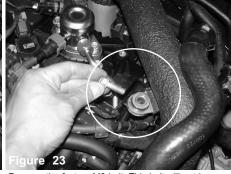
Remove the factory M8 bolt. This bolt will not be reused in this intake installation. A longer supplied M8x40 bolt will be used.
