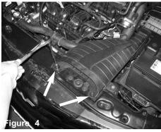
Use a 10mm socket/rachet and remove the two M6 bolts attached to the factory air box inlet duct.
