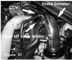
Re-attach all three vauum lines removed from figure 9. Re-install the engine cover The Blow off valve return, crank case breather and brake booster line will be re-attached.
