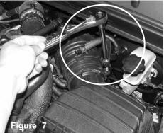
Loosen the clamp on the intake air duct connected to the air box assembly. Detach the intake air duct from the air box assembly
