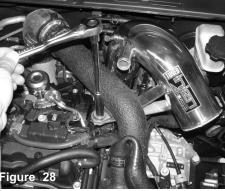
Use a 12mm socket/rachet to secure the Injen intake bracket to the factory upper intercooler pipe bracket
