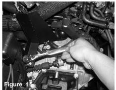
Use a 10mm socket/rachet and tighten the bolt
