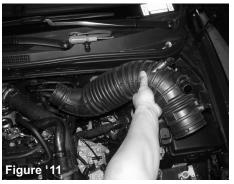
Detach the intake air duct from the turbocharger and you may now remove the intake air duct from the engine bay.
