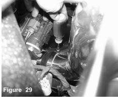
Once you have positioned the Injen intake pipe for best fitment, continue to tighten the #48 clamp on the 3.00" side of the step hose on the turbocharger securing the pipe to the step hose.
