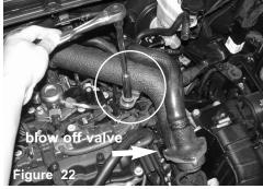
Loosen the M8 bolt with a 12mm socket/rachet on the upper intercooler piping next to the factory blow off valve.
