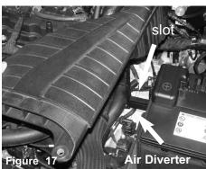
Re-install the inlet duct and make sure the slot of inlet duct lines up with the slot on the air divert. Arrow indicates air diverter and slot indicated in figure 16
