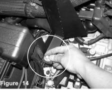
Place a M6x16 bolt and a fender washer onto the air diverter and attach it to the threaded hole.
