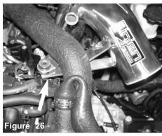
Injen intake bracket shown under factory upper intercooler pipe bracket
