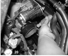
Use a 8mm nut driver and only tighten the #40 clamp on the 2.50" side of the step hose attaching the step hose to the turbo inlet
