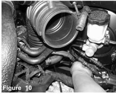
From the bottom side of the intake air duct, loosen the clamp with a 10mm socket/rachet attached to the turbo inlet.
