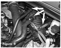
Use a plier and loosen and pull back on the three pressure clamps. The crank case breather line, blow off valve return line and brake booster line will be detached from the intake air duct.
