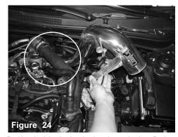
Position the Injen intake pipe into the engine bay. Push the  $3.00^\circ$  end of the pipe into the  $3.00^\circ$  end of the step hose already on the turbocharger inlet from figure 20
