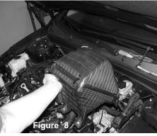
You may now pull the entire air box assembly out of the engine bay by lifting up and out.
