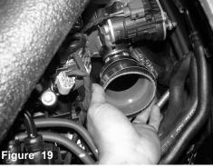
Install the 2.50"-3.00" step hose with 1-#48 and 1-#40 clamp onto the inlet of the turbocharger compressor inlet. The 2.50" end goes onto the turbocharger inlet
