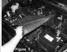
Remove the air box inlet duct from the engine bay. This air duct will be re-used in this installation to draw in cool air to the Injen intake system.
