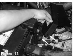
Behind the battery, Align the hole on the Injen air diverter with the pre-threaded hole where the left bolt that once attached the factory air box assembly too.
