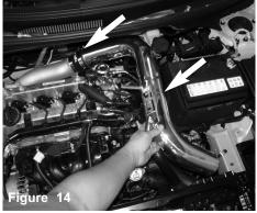
Position the intake pipe into the engine bay and place the end of the pipe into the step hose on the turbo compressor outlet.
