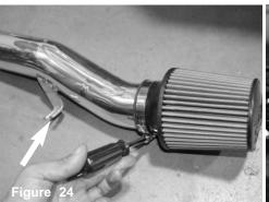
Place the filter onto the end of the secondary intake tube. Reference the intake bracket in the photo to locate the end of the pipe.
