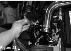
To continue with the installation of the cold air intake system, you will have to remove the filter and replace it with a 3.0" straight hose and two #48 clamps
