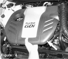
Firmly lift up on the engine cover and remove the engine cover from the engine bay.
