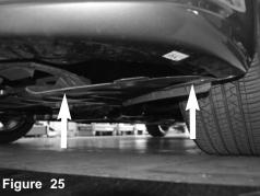
Unscrew the two screw to the access panel underneath the drivers side bumper. Pull the access panel bacn to gain access to the bumper cavity. The intake pipe and filter will be installed through here.
