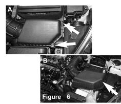
*Figure A:* Unclip the two tabs from the lower air box assembly to the upper air box assembly. *Figure B:* Detach the upper air box assembly from the lower assembly
