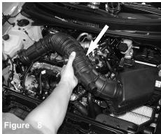
Remove the entire upper air box assembly and air duct from the engine bay
