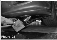
Insert the secondary pipe with the filter already installed from figure 25
