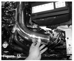
Line up the intake bracket to the vibra mount in figure 13
