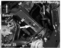
Screw the second vibramount mount into the threaded hole located on the chassis beneath the back of the driverside headlight housing inside the engine bay. Use the headlight housing and battery location in the photo for reference
