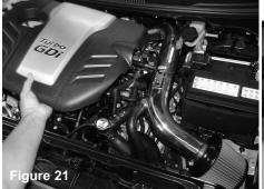
Reinstall the engine cover. Your short ram intake system installation is now complete. Go over all your clamps and fittings to make sure they are snug. Check the clearance on the pipe and make sure it does not make contact with any components in the engine bay.
