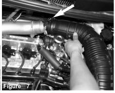
Use a 10mm socket and rachet and loosen the 10mm clamp bolt on the air duct located on the Turbo charger compressure outlet. Pull the air duct from the outlet.
