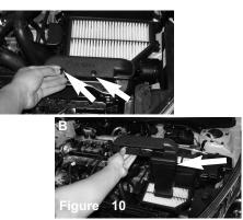
Figure A: Use a phillips screw driver and remove the two plastic screw clips from the front air intake duct Figure B: Lift up and remove the front air intake duct
