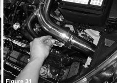
Adjust the entire intake system for best fitment. Make sure the intake pipe and filter does not come into contact with any objects and then continue to tighten the clamps on the 3.0" straight hose attached to the primary and secondary pipes.
