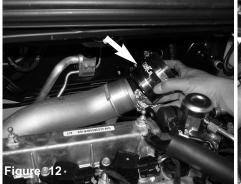
Place the 2.75"X3.00" step hose, #40 and #48 clamp onto the turbocharger compressor outlet.
