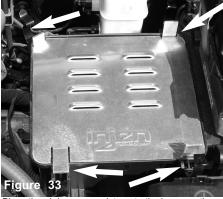
Place the air box cover plate onto the lower portion of the air box. The four arrows indicate mounting points
