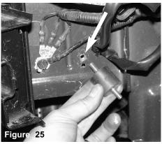
Place the vibramount onto the pre-threaded hole the right ground wire was once located.
