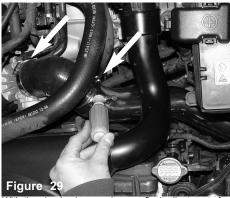
With the pipe in place, make your final adjustments for the best fitment and then tighten both clamps on the 90 deg. elbow located on the throttlebody.
