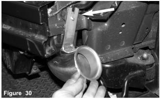
With the intake pipe in place, make sure the lower intake bracket lays flush with the vibramount
