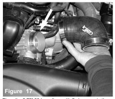
Place the 2.75" 90deg. elbow with 2 clamps onto the throttlebody. Make sure you have the long end of the 90 deg. hose on the throttlebody side.
