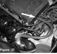
Place the 17"-10mm vacuum hose over the breather port under the engine cover.
