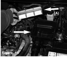
Remove the air filter element. (A) Lower portion of the air box will be retained to keep the ECU cool
