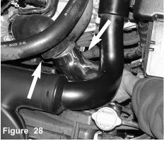
Slide the intake pipe from the bottom and work the pipe into the 90 deg. hose already located on the throttlebody.
