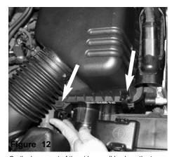
On the lower part of the airbox, pull back on the two retaining clips holding the top of the air box to the lower portion of the airbox
