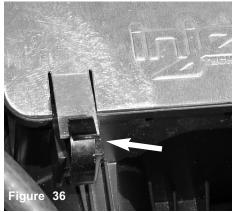
Place the retaining tab over the horizontal tab.
