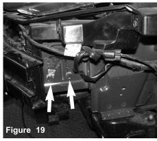
Locate a set of ground wires located under the drivers side headlight, behind the bumper support.
