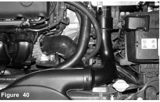
Vacuum line installed on pipe
