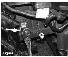
Now loosen the 10mm bolt securing the left set of ground wired
