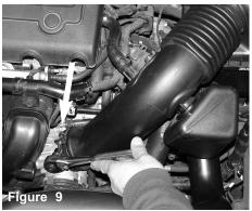
Loosen the throttle body clamp as shown above.
