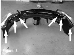
Bumper shown removed from vehicle showing 6 additional clips that will need to be removed from the bottom.
