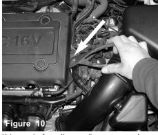
Using a pair of needle nose pliers, compress clamp on the crank case port underneath the engine cover and pull the clamp back.
