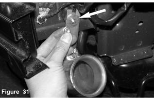
Place the fender washer and the M6 flanged nut over the bracket.
