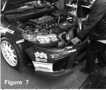
Once all plastic clips and screws have been removed continue to pull the front bumper off
