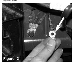
Ground wire that needs to be relocated shown above
