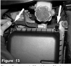
Now on the upper part of the air box, pull back on the retaining clips.  $\,$
