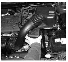
With all four retaining clips loose, remove the entire upper portion of the air box and air duct.
