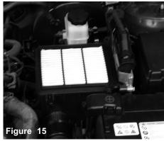
Once the upper portion of the air box is removed, you now have access to the air filter element.
