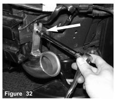
us a 10mm socket and rachet and tighten the M6 nut to the bracket
