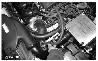
Now place the other end of the 10mm vacuum hose over the welded nipple on the intake pipe.
