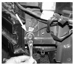
Now tighten the 10mm bolt to the frame
