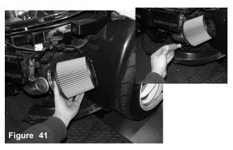
Place the filter on the end of the pipe and then tighten clamp on filter
