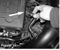
The clamp on the crank case has been pulled back, now continue to pull the breather hose off the crank case port.
