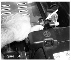
Press the factory air box retaining clip over three air box cover tabs.
