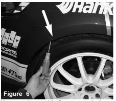
Unscrew and removed the 8mm screw under the passanger and driver side wheel well.
