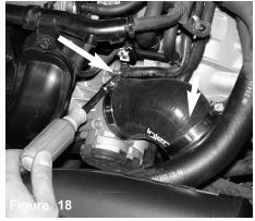
Now snug the clamp on the throttlebody side, make sure you leave it slightly loose to make some adjustments later
