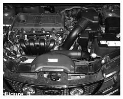
Stock air box cleaner and air ducts shown in this picture. Before getting started with the installation, be sure to disconnect the negative battery terminal.
