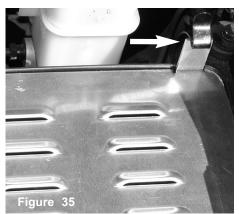
Close up photo showing retaining clip on air box cover tab
