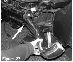
The intake pipe will be inserted from the bottom, behind the bumper support.
