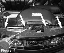
Loosen and remove the four plastic clips from the front shroud cover.
