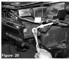
Loosen and remove the 10mm bolt on the right ground wire only. This wire will be relocated to the set of ground wires on the left.
