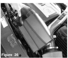
Remove the 2 screws holding in Stock ram air unit. Remove the ram air unit. Save the screws for new Injen power-ram scoop install.
