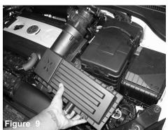
Pull out the complete air box assembly.
