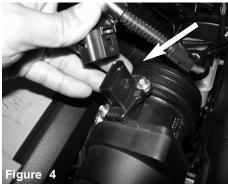
Disconnect MAF sensor harness and set aside.
