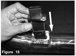
Install the MAF sensor to the intake tube.
