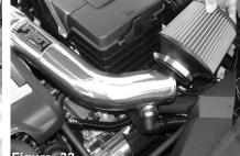
Tighten the screws using t25 torx bit.
