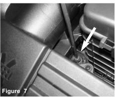
With T30 torx bit, loosen the screw holding in air box.
