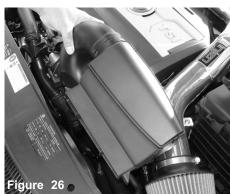
Remove the 2 screws holding in Stock ram air unit. Remove the ram air unit. Save the screws for new Injen power-ram install.
