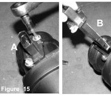
A) With T20 security bit loosen the 2 screws holding. B) Remove MAF sensor.
