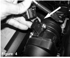
Disconnect MAF sensor harness and set aside.
