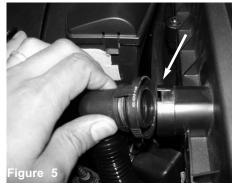
Pinch the harness on smog pump and pull away from air box. (if equipped with smog pump)
