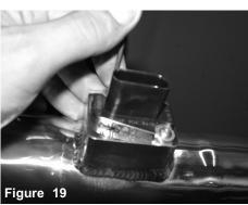
Secure the MAF sensor to tube using provided M4 screws and tighten using 2.5mm allen key.
