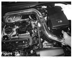
Install the intake tube into vehicle and position to turbo and bracket to vibra mount.
