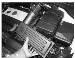
Pull out the complete air box assembly.
