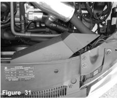
Make sure the power-ram is secure and tighten.
