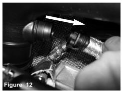
Pinch and pull back crank case line from intake tube.
