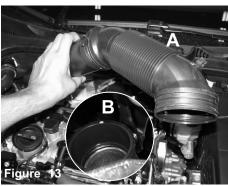
A) Remove intake tube out of vehicle.
