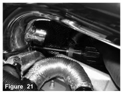
Tighten the remaining clamp on step hose using 8mm nut driver.
