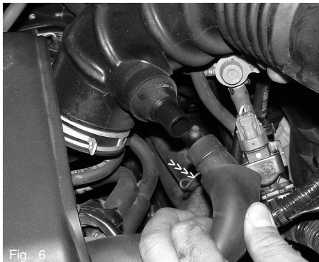
Fig. 6 Use a pair pliers to depress the wire tension clamp located on the crank case breather hose. Pull the breather hose off the air intake port as shown above.
