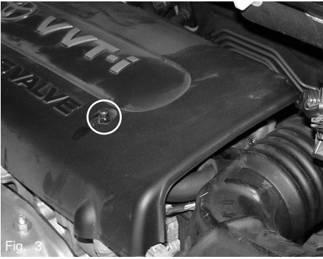
Fig. 3 Remove the engine cover that is secured by two 6mm acorn nuts.
