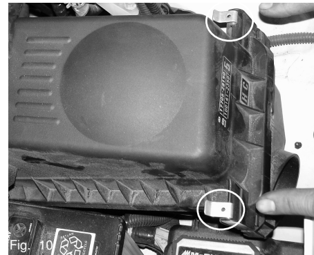
Fig. 10 Pull the two metal clips off the lower box pins and separate the air box top from the air box bottom.
