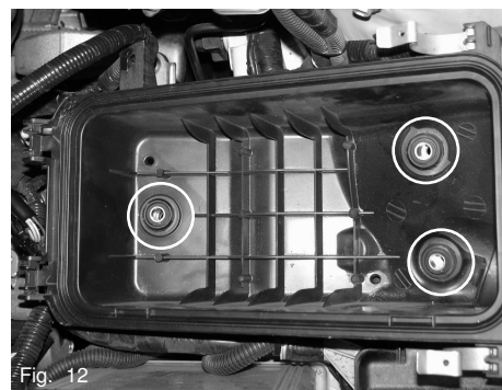
Fig. 12 Unscrew and remove all three bolts from the lower air box cleaner. Continue to remove the remaining fender well plastic air inlet duct, not shown in this picture.
