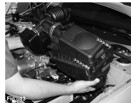
Fig. 13 Replace the air box top and re-attach the metal clips as shown above. Remove the entire air box cleaner and air intake duct as shown above.
