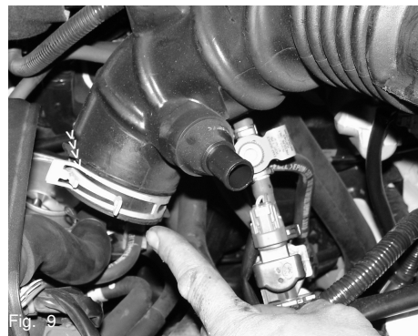
Fig. 9 Use a pair of pliers to depress the metal tension clamp while the air intake duct is pulled off the throttle body as shown above.
