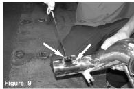
Place the MAF sensor into the MAF sensor adapater on the Injen intake pipe. Use two supplied M4 screws and secure the MAF sensor to the adapter with a 2.5MM allen
