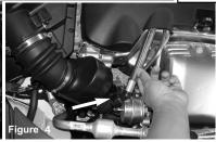
Use a flat head screw driver to release the retaining clip on Use a 8mm nut driver and loosen the clamp on the turbo the crank case ventilation breather line connected to the factory turbo duct. Lift up and disconnect CCV line from the
