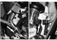
opening. Figure B: Run the MAF sensor harness under the heatshield and then connect the harness to the MAF
