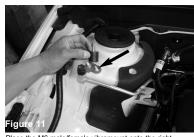
Place the M6 male/female vibramount onto the right (The stud without the factory nut)
