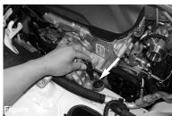
Place the supplied M6 Stand Off Stud onto the factory lower air box grommet
