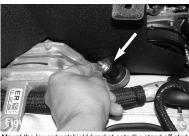
Mount the lower heatshield bracket onto the stand off stud from figure 10. Then place a washer and a M6 nut onto the stand off.
