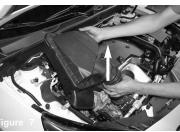
Firmly lift up on the factory air box assembly until the air box detaches from the mounting grommets
