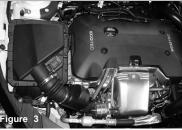
Stock air box assembly shown in this picture. Disconnect battery before the install.
