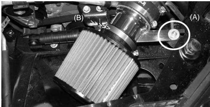
Take the 6mm flange nut and fender washer and secure the intake bracket to the vibra-mount stud (A) Press the filter over the end of the secondary intake and tighten the filter neck clamp (B).
