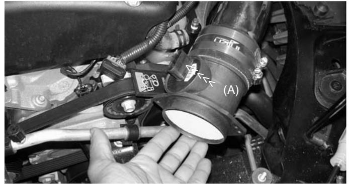
Take the directional mass air flow sensor and press the outlet end into the 3 1/8" hose located on the primary intake. Locate the female harness connector facing the firewall (A).
