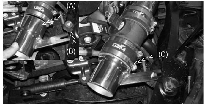
when using the short ram, press the secondary step intake and press the 3 3/8" end into the mass air sensor hose (A). Align the intake bracket to the vibra-mount stud (B). Once the bracket has been aligned adjust the intake for best fit and tighten the clamp on the mass air flow sensor (C).
