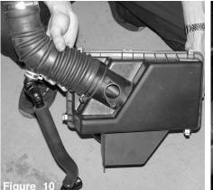
The entire air box cleaner and air intake duct are pulled up and out of the grommets. Page 2 of Part# SP6071
