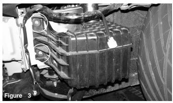
Once the bumper has been removed, continue to remove the three bolts holding the air resonator box to the frame. Two bolts are shown in this picture.
