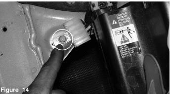
Remove the bolt that grounds the wire connectors to the frame. This is where the vibra-mount will be placed.
