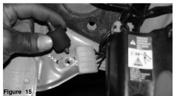
The vibra-mount is aligned and screwed into the existing pre-threaded hole.
