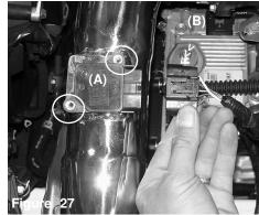
The stock screws are used to fasten the mass air flow sensor to the adapter (A) . Press the electrical harness over the mass air flow sensor until they have snapped together (B).
