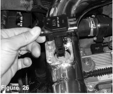
Insert the mass air flow sensor into the machined adapter. Use a a dab of light oil on the O-ring to insure good fitment and seal.
