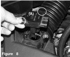
Remove the two screws from the mass air flow sensor (A) then pull the mass air flow sensor out from the sensor housing (B).
