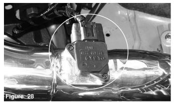
The bolts have been fastened to the sensor adapter and the electrical harness is firmly placed over the mass air flow sensor.
