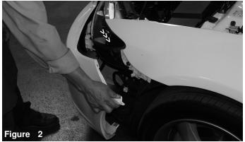
Remove all plastic clips and screws securing the bumper to the fender and radiator shroud. Once the bumper has been detached, continue to remove the front bumper for easy access to the resonator box.
