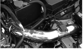
Congratulations! You have just completed the installation of this cold air intake system. Periodically, check the fitment of this intake system to avoid shifting of the intake that may damage the intake from rubbing and hitting of metal parts.
