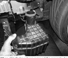
When all bolts have been removed the resonator box will detach itself from the frame.
