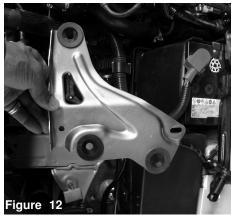
Once you have removed the two bolts continue to pull the brace out of the engine compartment.
