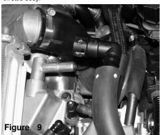
Depress clip on the ventilator hose coupler and pull the coupler out from the crankcase port. The hose and coupler will stay intact with the air box cleaner.
