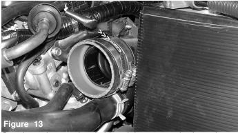
Press the step hose over the turbo inlet and place two power bands over the hose. Tighten the power band located over the turbo inlet for now.
