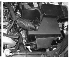
The stock air box is now ready to be pulled out of the engine compartment. The clamp over the throttle body is loosened to disconnect the air duct from the throttle body.
