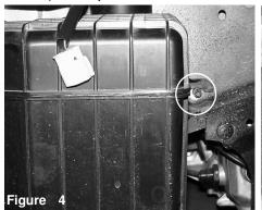
The third bolt is shown on the air resonator box to be removed.
