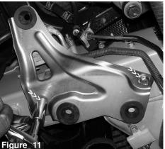
Remove the two bolts that fastens the air box brace to the frame.
