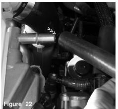
The 15mm hose is pressed over the crankcase venti-
