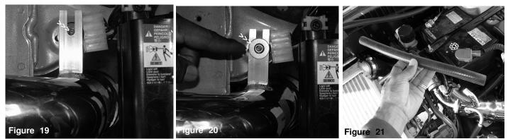
The intake bracket is aligned to the vibra-mount stud.
