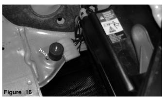
The vibra-mount is screwed in place until it sits flush over the connecter plate.
