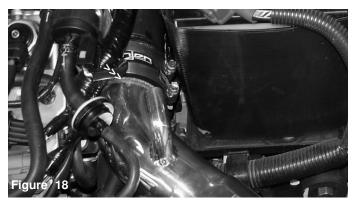
The top intake is pressed into the turbo hose inlet, while the intake bracket is aligned to the vibra-mount stud.
