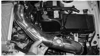
Lower the intake into the engine compartment, align the top end to the inlet hose and the intake bracket to the vibra-mount stud.
