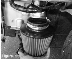
Press the filter over the intake end. The filter will come to a stop when the stops have butted up against the intake end, tighten the filter clamp.
