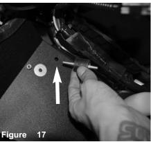
Secure the other hole using provided Long stud vibramount, install the long side first. Secure using fender washer and locknut.
