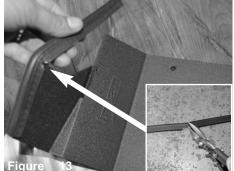
Install the bulb trim to the top of the heatshield. Cut the corner and notch a V for a clean cut and bend.
