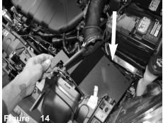
Now install the straight hose with clamps on the turbo. Tighten the clamp on the turbo side only.
