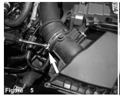
Loosen the clamp on the air box using 7mm nut driver. Pull back the ram air scoop from radiator support.
