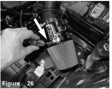
Secure the filter using 8mm nut driver.
