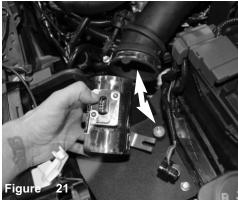
Install the intake tube and position the bracket to the vibramount. Install tube into the stock intaket tube.
