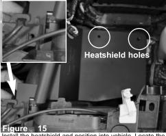
Install the heatshield and position into vehicle. Locate the 2 holes on heatshield to the grommets. Locate the tab on heatshield and slide under the factory plastic radiator support.
