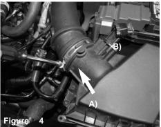
Loosen the clamp on the air box using 8mm nut driver.
