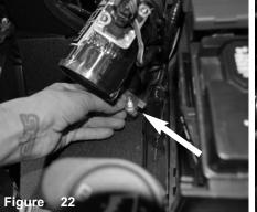
Secure the bracket using provided M6 nut and fender washer.
