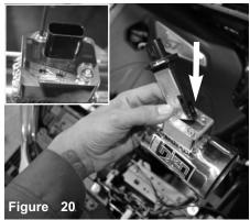
Now install the MAF sensor into the new intake tube and secure and tighten using provided M4 screws.
