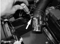
Secure the intake tube and tighten using 7mm nut driver.
