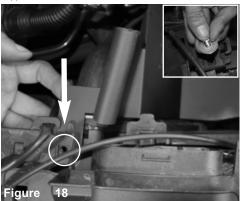
Locate the tab on heatshield and slide under the factory plastic radiator support. Secure the front tab using provided M6 screw and fender washer
