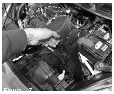
Now lift up and remove the stock air box out of vehicle.
