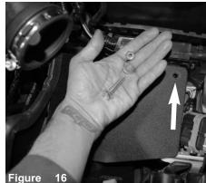
Secure the this hole on heatshield using provided Long M8 bolt, secure back side using washer and M8 locknut.
