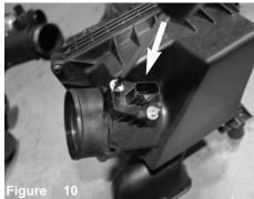
Loosen the 2 screw holding in the MAF sensor using T20 torx bit. Carefully remove MAF sensor from air box.
