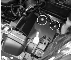
Install the heatshield and position into vehicle. Locate the 2 holes on heatshield to the grommets. Locate the tab on heatshield and slide under the factory plastic radiator support.
