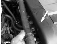
Pull back the diverter tube from air box/engine cover.
