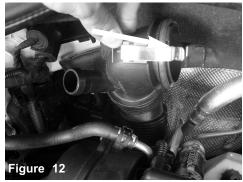
Pinch the clamp on the turbo and remove the intake tube.
