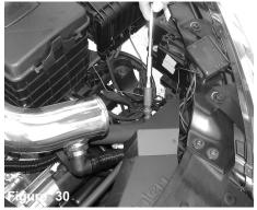
With adjustable torx snake, tighten both screws.
