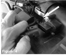
Disconnect MAF sensor harness and set aside.
