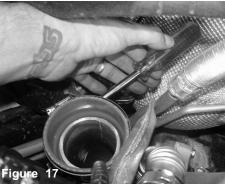
Install the step hose to the turbo with clamps Tighten the clamp on the turbo only using 8mm nut driver.
