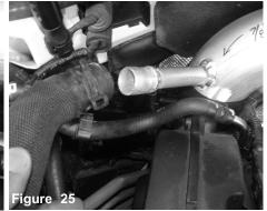
Attach the diverter valve hose to the fitting on the intake tube.
