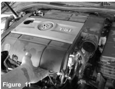
Lift up and remove the air box/engine cover from the vehicle.
