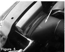
Loosen the 2 bolts holding in the Ram scoop, using T25 torx bit.
