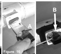
A) Install the MAF sensor into the the new intake system.
