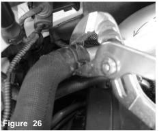
Secure the hose using the factory pinch clamp.
