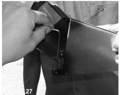
With screw, install and hold with torx key.
