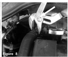
With pliers, carefully pinch clamp and pull intake tube away from air box.
