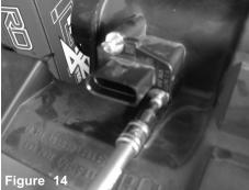
With T20 security bit loosen the 2 screws holding in the MAF sensor.
