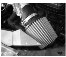
Install the filter and secure using 8mm nut driver.
