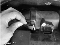
Un-clip the intake tube to from the air box/engine cover.
