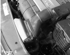
Pull out ram air assembly from vehicle.
