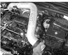
Install the intake tube into vehicle and position to turbo and bracket to vibra mount.
