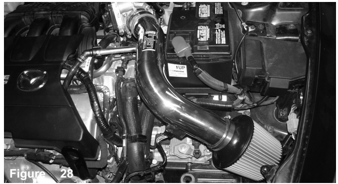
Align the entire intake for the best possible fit. Once you have rechecked and cleared the intake from all moving parts, continue to tighten all nuts, bolts and clamps.
