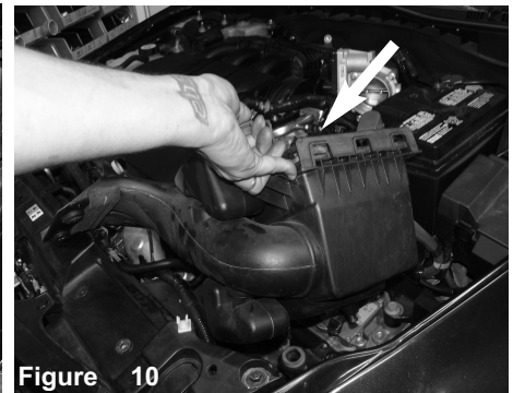
Figure 10 Lift up and remove the lower air box assembly.
