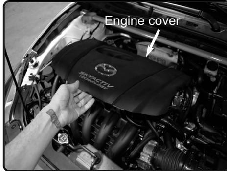
**2.** Lift up and remove engine cover.
