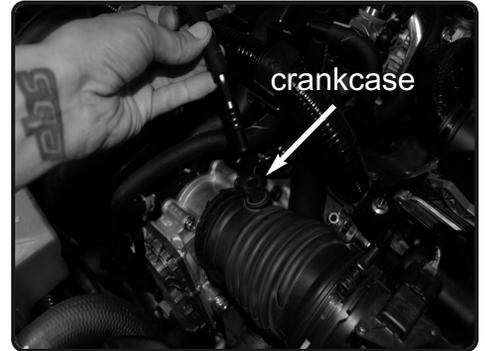
**3.** Lift up and remove the crankcase line from intake tube.
