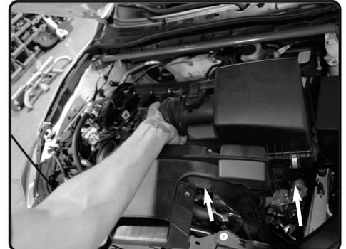
**7.** Lift up and remove the complete stock intake system out of vehicle.
