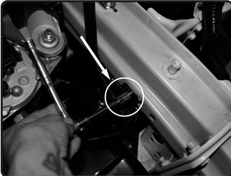
**12.** Locate the Harness bracket, loosen the 10mm screw. This is where the Heatshield will be mounted to. Save screw for later install.
