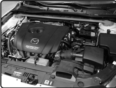
**1.** Stock intake system shown. Disconnect battery, vehicle may throw Check Engine Light if not disconnected. MAF sensor has constant voltage running even with vehicle off.
