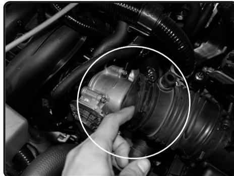
**6.** Pull back the intake tube from the throttle body.
