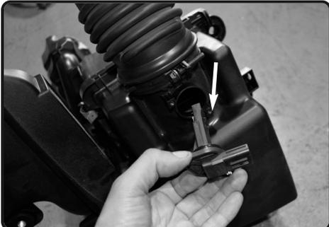
**8.** Loosen and remove the MAF sensor out of air box using phillips screwdriver.
