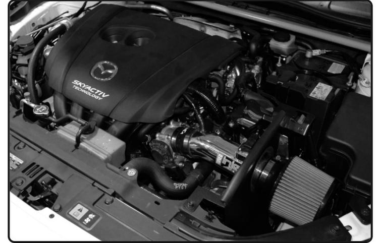
Congratulations! You have just completed the installation of this intake system. Periodically, check the alignment of the intake, normal wear and tear can cause nuts and bolts to come loose.
