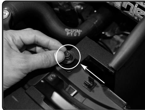
**18.** Secure the tab of the heatshield using Original screw from Air box. Do not tighten.
