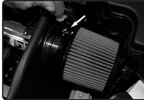
**25.** Install the filter to the intake tube, secure and tighten using 8mm nut driver. Re-install engine cover. Re-connect battery.
