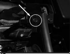
17. Secure the ECU bracket of the heatshield using Original screw from ECU bracket. Do not tighten.
