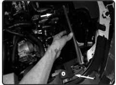
**14.** Position the heatshield into the vehicle, Do not secure.
