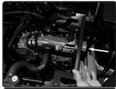
**15.** Now install the intake tube into the vehicle. Make sure the hose is on the throttle body. Do not tighten.
