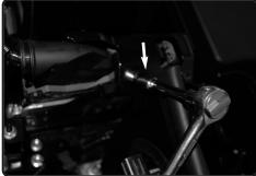
**21.** Tighten the ECU bracket using 10mm socket or wrench.
