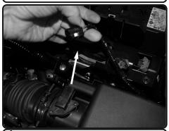
**4.** Disconnect MAF sensor harness and pull away from airbox.
