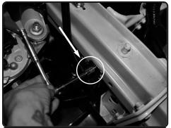
**12.** Locate the Harness bracket, loosen the 10mm screw. This is where the Heatshield will be mounted to. Save screw for later install.
