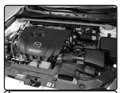
1. Stock intake system shown. <u>Disconnect battery</u>, vehicle may throw Check Engine Light if not disconnected, MAF sensor has constant voltage running even with vehicle off.
