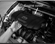
2. Lift up and remove engine cover.
