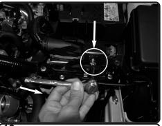
**13.** Loosen the the screw on the ECU bracket. This is where the Heatshield tab will be mounted to. Save screw for later install.
