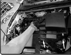
7. Lift up and remove the complete stock intake system out of vehicle.
