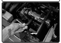
**20.** Tighten tab using 10mm socket or wrench.
