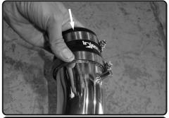
**10.** Install the step hose with clamps provided to the intake tube. Do not tighten.
