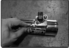
**9.** Secure and install into the new injenintake tube using M4 screws. Tighten using 2.5mm allen key.
