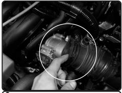
**6.** Pull back the intake tube from the throttle body.
