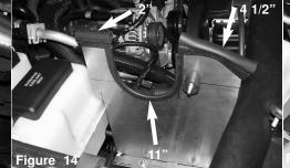
the 2" on the upper left and the 11" Vinyl trim on the U shape opening on the heatshield
