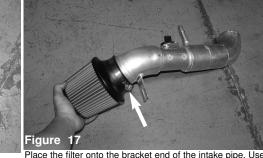
a 8mm nut driver to secure the filter clamp onto the welded MAF sensor adapter welded on the Injen intake pipe. Then secure the screws with a 2.5mm Allen
