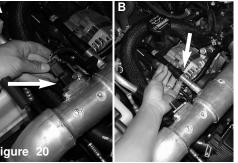
Figure A: Reconnect the MAF sensor harness to the MAF sensor *Figure B:* Connect the crank case vent tube to the machined nipple on the intake pipe. Make sure you hear a click indicating a secure fit and seal
