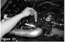
Make sure the intake pipe, filter and heatshield doesn't come into contact with anything and then make your final adjustment before securing the last clamp on the throttlebody.
