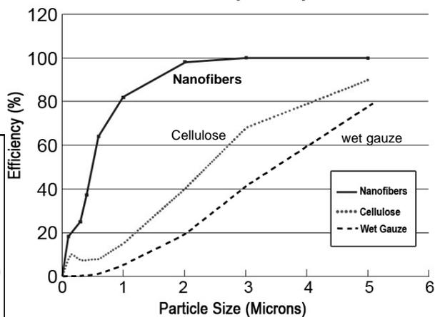
**Nanofiber technology:** Is an oil free filtration media that has been used exclusively in heavy duty applications, including the US Army's Abrams M1 tanks.
