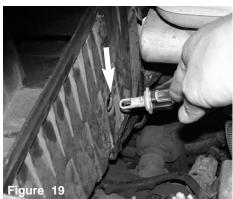
The air temperature sensor is now pulled away from the air box as shown above.
