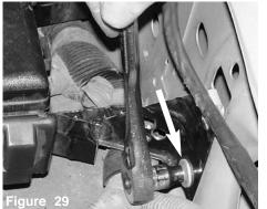
The third bolt is loosened and removed
