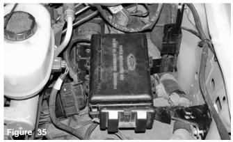
The large relay box is installed on the stand-offs. The relay box sits lower and the fuse box by the fender well.
