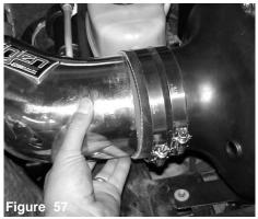
Once you have inserted the lower end into the step hose, continue to insert the inlet side into the plenum hose.
