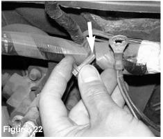
The 10mm ground screw is now removed. Note, the screw will be reused later in the instructions.
