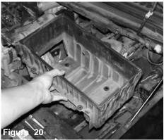
The lower air box cleaner is now ready to be pulled out of the engine compartment.
