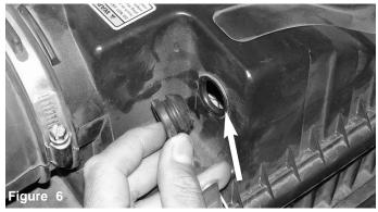
Once the restrictor gauge has been removed, continue to pull the grommet out out of the air box.
