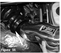
The case aluminum intake is slipped into the turbo hump hose.
