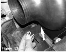
The remaining two m6 bolts are screwed into the heatshield bottom press nuts.
