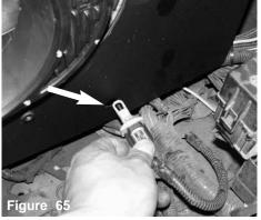
The air temperature sensor is lined up to the stamped hole.
