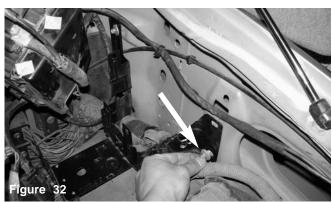
The new relay bracket is aligned to the bolt pattern and the stock bolts are used to re-attach the bracket.
