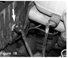
The air temperature sensor will be removed from the lower air box cleaner.
