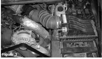
The stock air box cleaner and air duct to be removed.
