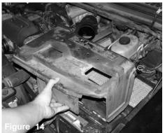
Once you have removed the battery terminals, continue to pull the battery cover away from the battery.
