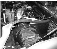
.The 18" foam vinyl trim is pressed along the edge of the heat shield as shown above
