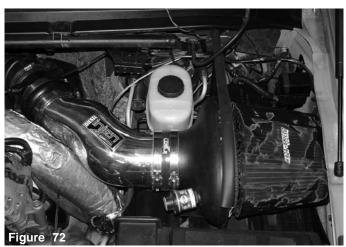
Check the entire system for the best possible fit. Once you have checked the entire system for leaks, rubbing or rattling, continue to tighten all nuts, bolts and clamps. Reconnect the negative battery terminal prior to starting the engine.
