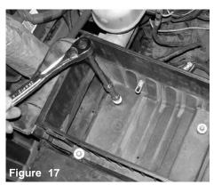
The 10mm bolts are now being loosened and removed
