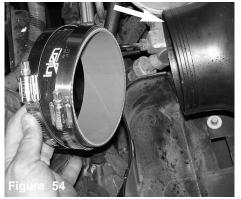
The 4 1/2" straight hose is slipped over the end of the plenum. A small amount of light oil maybe needed to slip the hose over the plenum.
