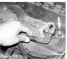
Loosen the negative battery terminal and remove the terminal from the battery post.
