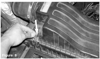
Unlatch the first metal clamp from the upper air box as shown above.
