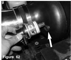
The restrictor gauge is carefully inserted into the grommet.
