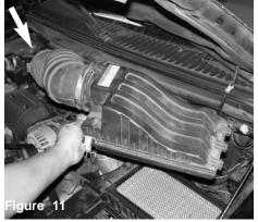
Pull the air intake duct from the turbo inlet then pull the entire upper assembly out of the engine compartment.
