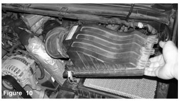
Once you have unlatched the metal clamps from the upper air box continue to separate the upper air box top from the lower air box.
