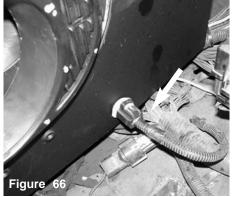
The electrical harness is inserted in the heatshield stamped hole.
