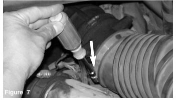
Loosen air duct clamp over the turbo inlet hard pipe. The air intake duct will be removed from the turbo inlet.
