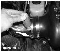
The clamp over the inlet side is tightened.
