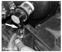
The electrical harness is pressed over the restrictor gauge male plug.
