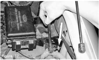
The second lower bolt to located to the front is also tightened as shown above.
