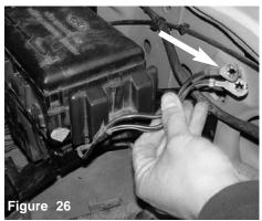
The ground wire is shown removed from the driver side fender well.
