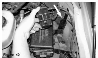
The small fuse box is pressed over the single stand-off by the fender well.
