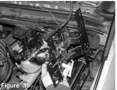
The stock relay bracket is ready to be pulled out of the engine compartment.
