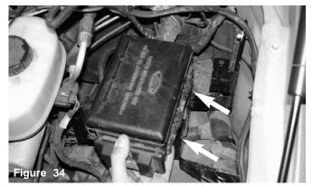
The large relay box is aligned to the stand-offs, two on each side, then pressed down onto the stand-offs.
