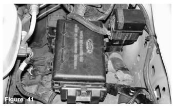
The new bracket is now installed and both fuse/relay box are re-installed.
