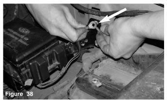
The front upper upper bolt is aligned over the ground wires and to the fender well.
