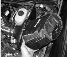
The hyrdro-shield is slipped over the Injen/AMSOIL filter, once you have fitted the hydro-shield, continue to press the filter over the velocity stack.
