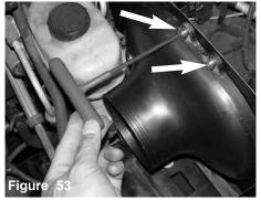
A 6m allen is used to torque the m6 bolts to the heat-shield.
