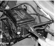
The bolt with the ground wire is loosened prior to removing the ground.
