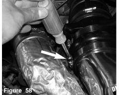
Adjust the entire cast intake for best fit then continue to tighten the clamp over the intake.
