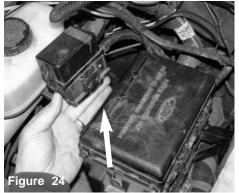
The small fuse box is dislodged from the stand-off located in front of the relay box.
