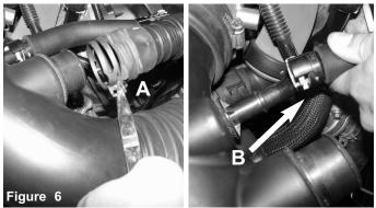
A) With pliers loosen the clamp holding in the sound tube connected at the intake tube and remove. Pull back sound tube. B) Disconnect crank case line from intake tube.
