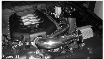
Check the entire system for the best possible fit. Once you have checked the entire system for leaks, rubbing or rattling, continue to tighten all nuts, bolts and clamps. Reconnect the negative battery terminal prior to starting the engine.
