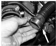
Make sure the OE clamp is removed, attach the new clamp to the sound tube.
