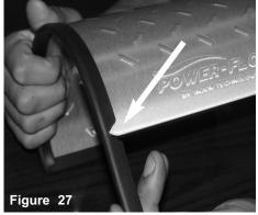
Provided vinyl trim can be installed to the edge of the heat shield. Cut a V out of the 2 corners to make the trim seal fit properly.
