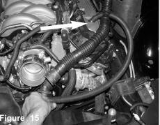
Install the 15mm hose to the engine fitting. Positon so hose sits under the intake tube.
