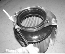
Install the filter to the center of the heat shield, place clamp around the brackets and postion, tighten clamp just enough to prevent the heat shield from coming off.
