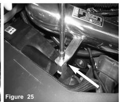
Secure the bracket using the provided M6 nut and washer. Tighten using 10mm socket and ratchet.
