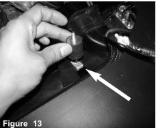
Install the M6 vibra mount to the thredded insert located on the radiator shroud.
