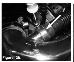
Install the sound tube to the fitting on the intake tube. Secure and tighten using 8mm nut driver.
