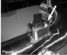
Secure the MAF sensor using 2.5mm button head screws. Tighten using allen key.
