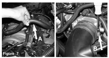
A) Disconnect crank case line from engine and remove from vehicle.B) Loosen the clamp on the throttle body using 8mm nut driver and pull back.
