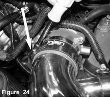
Tighten the clamps using 8mm nut driver.
