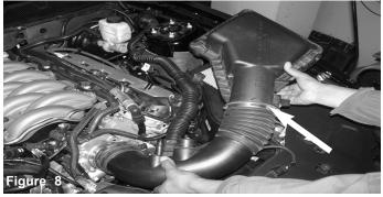
Carefully lift up and pull out the stock upper half of air box from vehicle.
