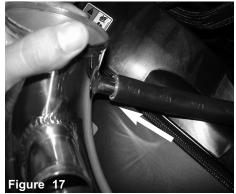
Attach the hose to the fitting on the intake tube.
