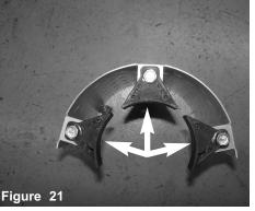
Take the heat shield, position like image above. Attach the brackets to the heat shield, secure the brackets using provided 5/16 hex screws and tighten.
