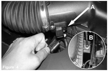
A) Disconnect the MAF sensor from harness.B) Loosen the 10mm bolt holding in the air box.
