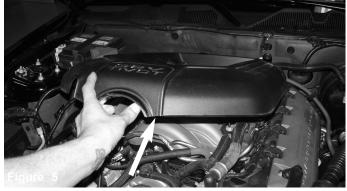
Carefully lift up and remove the engine cover.
