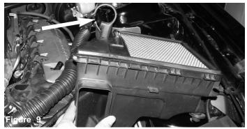
Carefully lift up and pull out the bottom air box from vehicle. Make sure that the sound tube rubber isolator is disconnected.
