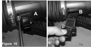
A) With T25 torx bit, loosen the 2 screws holding in MAF sensor. B) Carefully remove MAF sensor.
