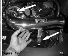
Position the intake tube to the throttle body and bracket to the vibra mount.
