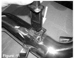
Install the MAF sensor into the intake tube.
