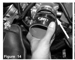
With clamps provided, install the 3-1/2" straight hose to the throttle body.
