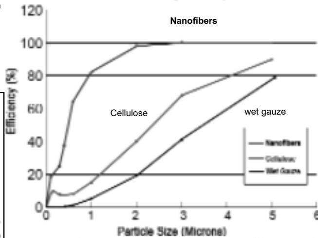
**Nanofiber technology:** Is an oil free filtration media that has been used exclusively in heavy duty applications, including the US Army's Abrams M1 tanks. Injen's is now making it available to diesel applications and vary soon will be available for the gas auto/light truck market
