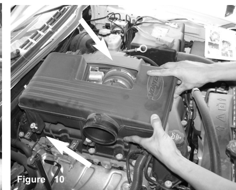
Figure 7 Once the air duct is removed from the air box resonator (Figure B) continue to remove entire air duct and air box cleaner out of the engine bay. (Figure A)
