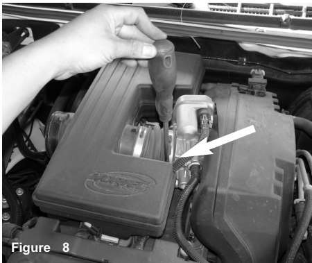
Figure 5 Once the 7mm screws have been removed, continue to remove the mass air flow sensor from the sensor housing.
