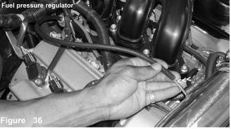
Press the 18" -4mm vacuum line installed earlier on the fuel pressure regulator over the 3/16 " intake port.
