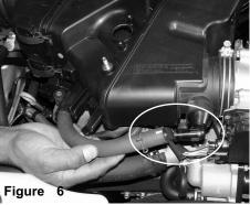
Unplug the crank case breather hose from the air box cleaner port as shown above.
