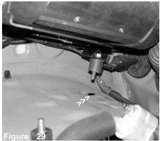
Lower the power box into the engine compartment, the rear vibra-mount fastened to the bracket is now inserted into the grommet hole location.
