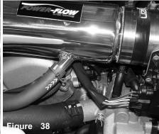
Once the breather hose has been properly installed over the  $5/8^{\circ}$  intake port, use the wire tension clamp to secure the breather hose in place.
