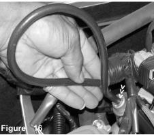
Press the 18 inch, 4mm vacuum line over the fuel pressure regulator port.
