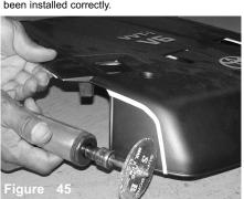
A grinding wheel or Dremel is recommended to make a clean cut along the line. A utility knife will also work but a file will be required to clean up the edge.
