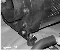
Once the rear vibra-mount is inserted into the rear grommet hole, use the m8 flange nut to fasten the bracket to the front vibra-mount.
