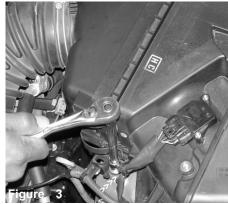
Unbolt the m6 bolt located on the grommet below the air box cleaner  $% \left( {{{\rm{D}}_{\rm{B}}}} \right)$
