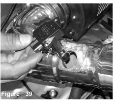
Rub a dab of light oil around the MAFS O-ring, then insert it into the sensor adapter. Be careful not to pinch the O-ring when inserting it into adapter.
