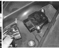
Unplug the electrical air sensor harness as shown above.
