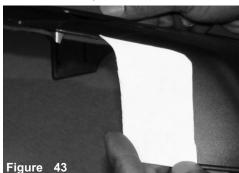
Take the sheet with the pattern and cut along the dotted lines. Use the pattern to place along the engine cover edge. The pattern is used as a guide to cut out a strip.
