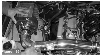
Now continue to insert the 4 inch intake end into the power box 4 inch straight hose as shown above (A) . Note the 1/4-20 stud placed over the intake (B) the stud must be facing up because this is where the engine cover will be attached.
