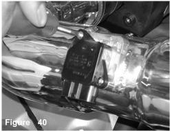
Use the two stock bolts to secure the MAFS to the machined sensor adapter.
