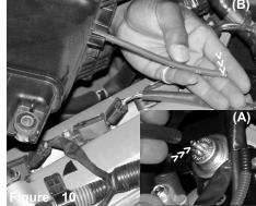
With all bolts lose, lift the entire air box cleaner and disconnect the 4mm vacuum hose on the fuel pressure regulator (A). The stock 4mm vacuum hose will remain on the air box cleaner (B).
