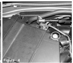
Remove the second m6 bolt that fastens the air box cleaner in place.
