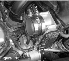
Press the 3" straight hose over the throttle body, install two power bands (.362) over the 3" hose and tighten the band located over the throttle body.
