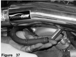
The stock breather hose is now aligned to the  $5/8^{\circ}$  intake firmly press the hose over the intake port.
