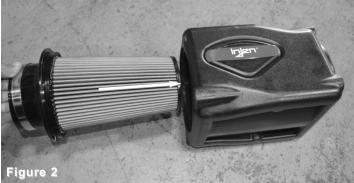
Install the provided Twist lock filter into the PowerFlow box.
