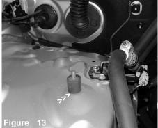
Screw the 3/8" side of the 8mm vibra-mount into the wheel well pre-tapped hole until the vibra-mount sits flush over the mounting point.
