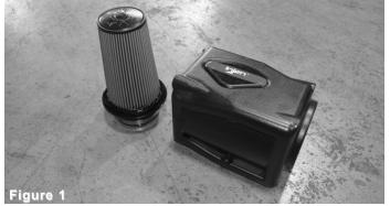
New Power flow box assembly. Twist lock filter and PowerFlow box. Box can be rotated to be either driver side or Passenger side fitment.
