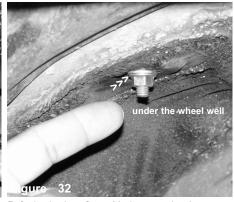
Referring back to figure 29, the power box is set on both vibra-mounts, a fender washer and an m8 nut will secure the vibra-mount inserted under the wheel well.
