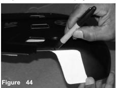
Place the pattern on the edge of the engine cover and use a marker to trace a line around the pattern.
