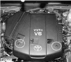
Loosen the two flange nuts located over the engine cover as shown above. Once you have removed both bolts, continue to remove the engine cover.
