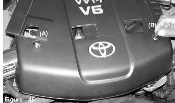
When the engine cover has been cut and fitted, lower the cover over the intake 1/4-20 aluminum stud(A) and intake plenum stud (B). Use one stack nut and 1/4-20 nut provided to secure the cover to the intake stud and the intake plenum stud.
