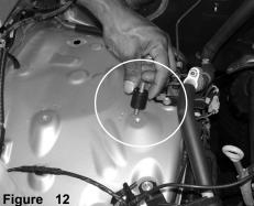
align the m8 vibra-mount to the pre-tapped hole located over the wheel well. For this installation, use the vibra-mount with the 3/8" stud x 5/8" stud, part#6067
