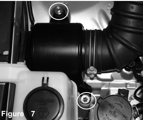
Figure 7 Loosen and remove the two m8 bolts that secures the resonator box to the fender well.
