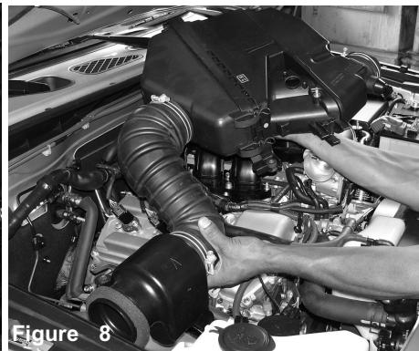
Figure 8 The entire air box cleaner and resonator box is now ready to be removed from the engine compartment.
