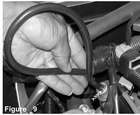
Figure 9 Remove the short 4mm stock vacuum hose from the fuel pressure regulator. Press the new 18 inch, 4mm vacuum line over the fuel pressure regulator port.
