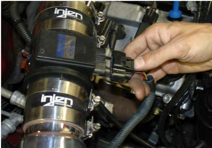
The sensor harness clip is reconnected. The harness is pressed over the air mass sensor until it snaps in place. When you hear the snap it usually means that the sensor and harness are properly secured.
