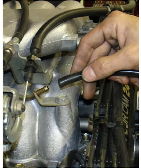
Use the 15" 6mm vacuum hose is pressed over the Fuel pressure regulator port as shown above. The fuel pressure regulator is located right below the throttle body.
