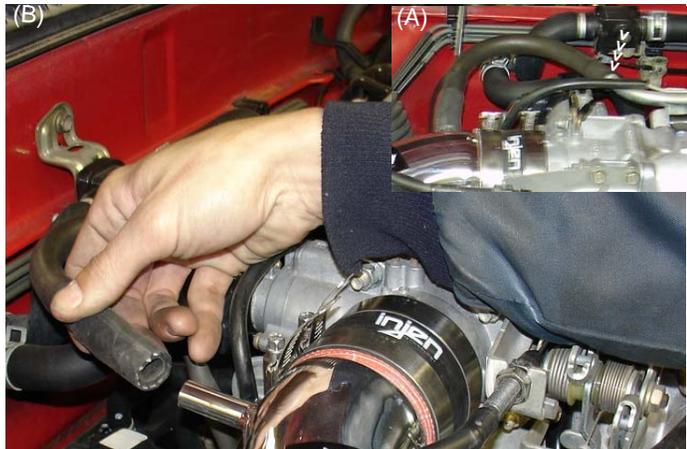
The stock crack case breather line is replaced with the 13" -10mm vacuum hose (A). Press one end over the crankcase breather port and connect the other end over the 1/2" intake port located by the firewall (B).
