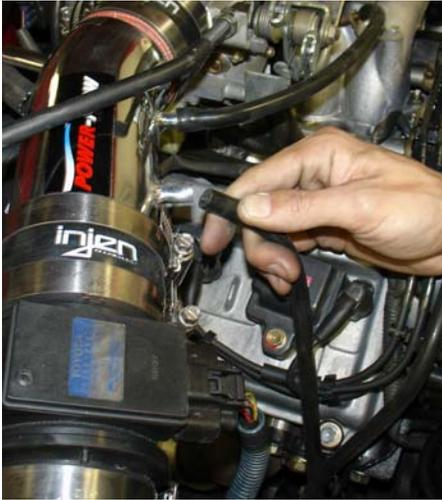
The 18"-6mm vacuum hose is pressed over the second intake port located on the primary intake. The other end lead down to the to Power steering switch port.
