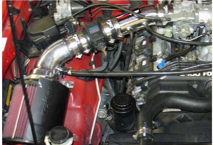
Congratulations! You have just completed the installation of the MR Tech intake system. Periodically, check the fitment of the intake system for safety precaution. Extra precaution will prevent possible damage to the intake system and or engine compartment. The Power-heat shield is sold separately on-line at [injenonline.com](http://injenonline.com)
