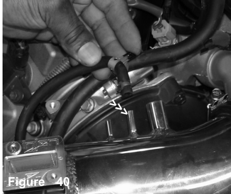
Figure 40 Press the stock 6mm hose over the center 3/8" intake port. Use the stock hose clamp to secure the line.
