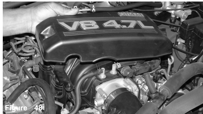
Figure 48 Align the engine cover to the intake bolt while lowering the cover over the intake. Use the 1/4-20 oval flange nut to fasten the cover to the intake threaded bolt. The engine cover will fit snug over the intake as shown above.
