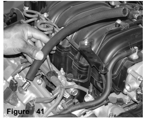
Figure 41 Press the 15"-15mm hose over the crank case breather port
