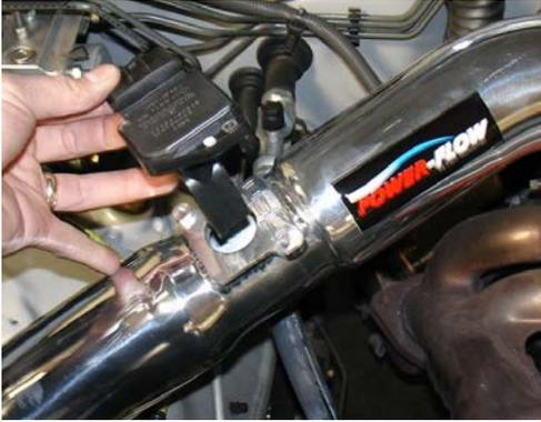
Take the mass air flow sensor and carefully insert it into the machined sensor adapter. we recommend you use a dab of light oil or water to wet the O-ring. This will allow the O-ring to slip into the hole for a better seal.
