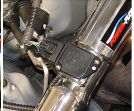
Take the harness clip and press it over the mass air flow sensor until you hear it snap in place, this will assure a good connection.
