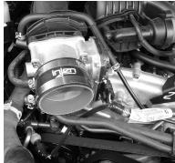
Place the 31/8 straight hose over the throttlebody and place twomedium (362) clamps over the hose, tighten only the clamp on the throttlebody side for now
