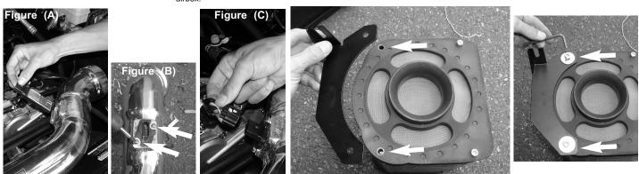
Place the MAF sensor onto the sensor pad on the Injen intake pipe. (Figure A) Re-use the two MAF screws to mount the MAF sensor on the sensor pad. (Figure B) Re-connect the MAF sensor harness, make sure you press firmly.
