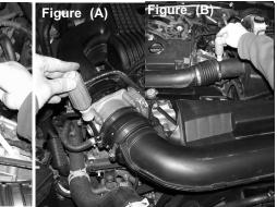
With both clamps loosened, remove entire air duct with the air resonator box attached.
