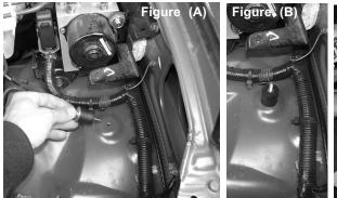
Place the vibramount ontp the pre-tapped hole located next to the ABS solenoid pump. (Figure A) Vibramount mounted on pre-tapped hole. (Figure B) This vibramount will be used for the mount point for the Injen airbox.
