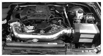
Check the alignment and fitment of the entire Power-Flow intake and Power box. Once you have check for possible air leaks, rubbing or rattling, continue to tighten all nuts, bolts and clamps.
