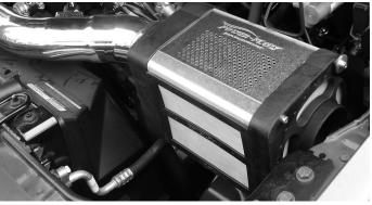
Here is a side view of the Power box installed and connected to the vibra-mount stud and air intake inlet.
