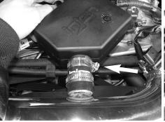
Press the CCV box over the large intake port, adjust and tighen clamp as shown in the picture.
