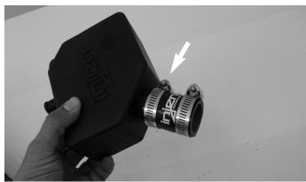
Once both clamps have been placed over the hose be sure to tighten the first clamp nearest to the CCV box.
