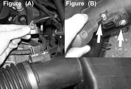
Unclip air mass sensor harness (Figure A) and then use a phillips screw driver to remove the two screws holding the MAF sensor to the housing. These screws will be reused.
