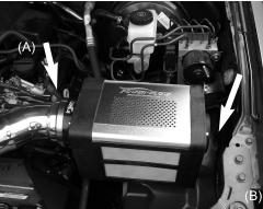
The four inch velocity stack base is connected to the ment and press four inch hose over the intake inlet intake (A) and the Power box bracket is lined up to the vibra-mount stud (B).
