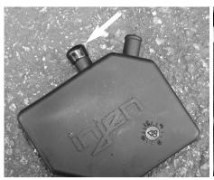
Press CCV box 5/8" vacuum cap over left port which will not be used.
