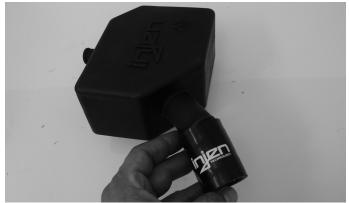
Take the CCV connecting hose and press it over the CCV box large port. Two clamps will be placed over the hose.
