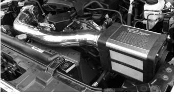
Congratulations! You have just completed the installation of the World's first tuned intake system, the Power-Flow intake, featuring MR Technology. Periodically, check the system for fitment, this will enhance the life of your Power-Flow system.
