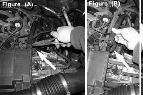
Loosen tension clamp with a plier. (Figure A) Then remove vacu- Use a 8mm nut driver to loosen clamp on throttleum breather line from air duct resonator box. (Figure B)
