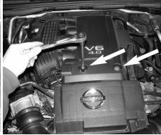
Use a 10mm socket with a 3/8 rachet and remove the two 10mm bolts on the engine cover.
