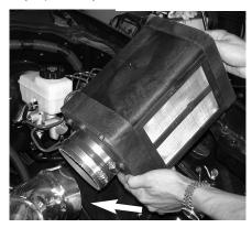
Postion Power-flow box in the engine compartas shown in this picture .
