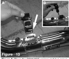
Figure A: Place the OEM MAF sensor and two srews into the billet MAF sensor adapter on the Injen intake pipe. Figure B: Use a phillips to tighten the screws to secure the MAF sensor to the adapter.
