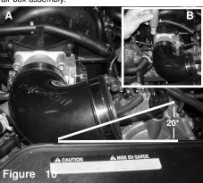
Figure A: Position the hose at 20 degee angle for the best position. Figure B: Use a 8mm nut driver and tighten the clamp on the throttle body side only for now.
