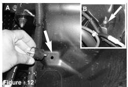
Figure A: Place the vibramount into the hole where the plastic retaining clip was removed from figure 11. Also place one M6 nut and fender washer on the bottom side of the wheel well cover to secure the vibramount to the wheel well with a 10mm socket and rachet. Figure B: Vibramount shown attached to wheel well
