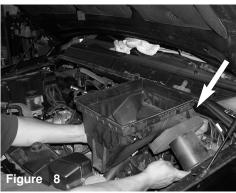
Remove the 10mm bolt on the back side of the lower air box assembly and then firmly lift up the air box assembly to detach it from the grommets and then remove from the engine bay.
