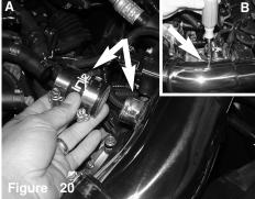
Figure A: Place the 1 1/8" hose with two #16 clamps onto the 1 1/8" welded nipple on the intakle pipe. Figure B: Only tighten the clamp on the welded nipple side for now.
