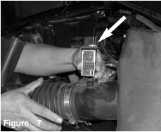
Use a phillips screw driver to remove the two screws from the MAF sensor. The MAF sensor and two screws will be reused. Now remove the entire upper air box assembly.
