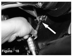
Use a 10mm wrench and tighten the M6 nut on the vibramount, securing the intake bracket to the vibramount
