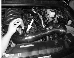
Adjust the intake pipe for the best fitment and then tighten the clamp on the 3.25"X3.50" elbow hose to secure it to the intake pipe.
