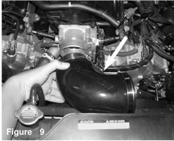
Place the 3.25"X3.50 Elbow hose and two #56 clamps onto the throttlebody with the 3.25" side on the throttlebody.
