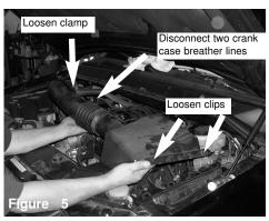
Use a 10mm socket and rachet to loosen the clamp on the throttle body. Then loosen the clips on the right side of the upper air box assembly. Then disconnect both of the crank case breather lines
