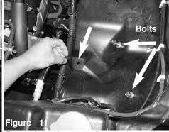
Remove the plastic retaining clip on the drivers side wheel well located in the original location of the OEM air box assembly. You can use the two remaining bolts once attached to the lower air box assembly grommets as a reference point.
