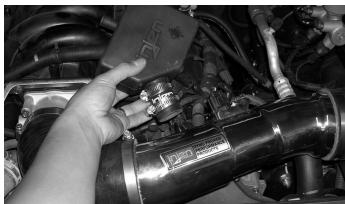
Take the assembled CCV box and press over the large port located on the
