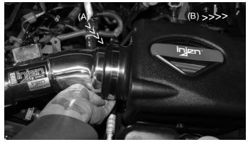
The Power box velocity stack base is connected to the intake (A) and the Power box bracket is lined up to the vibra-mount stud (B).
