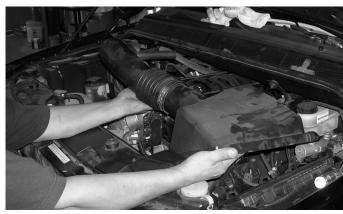
Remove screws, loosen clamps and remove upper air intake box and air intake duct connected to the throttle body.
