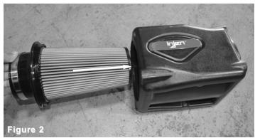
Install the provided Twist lock filter into the PowerFlow box.
