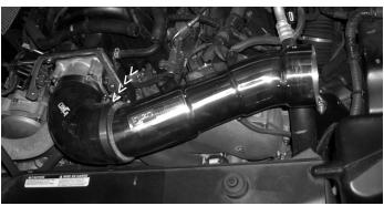
Take the assembled intake and press the  $3\ 1/2$ " end into the silicone elbow. Do not tighten clamp located on the silicone elbow.
