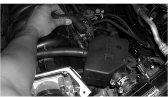
Locate the driver side breather hose and press it over the CCV box port as shown in this picture.
