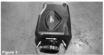
Once the filter is seated correctly and flat, rotate the filter 1/4" turn in either direction left or right and secure. Filter has built in lock.
