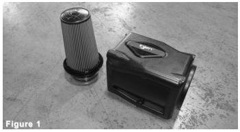
New Power flow box assembly. Twist lock filter and PowerFlow box. Box can be rotated to be either driver side or Passenger side fitment.
