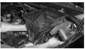
Remove flat filter panel from the filter box. Once filter has been removed, gently pull lower box out of the stock location.
