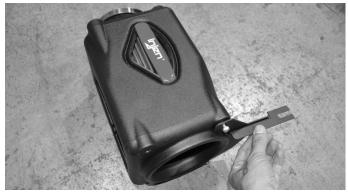
The bracket holes are lined up to the bolt pattern and the two M6 button head screws are used to secure bracket to air box. The bracket is now secured to the Power box.
