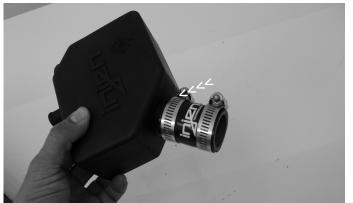
Take the CCV connecting hose and press it over the CCV box port. Use the two small clamps to hold the hose in place and tighten the clamp on the port side.
