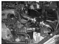
Reservoir tank relocated with bracket. >>>
