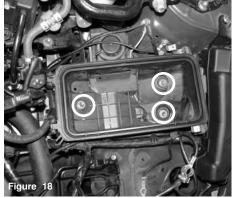
Once you have removed the upper air box cleaner, continue to remove the paper filter panel. Unscrew the three m6 bolts from the lower air box cleaner,
