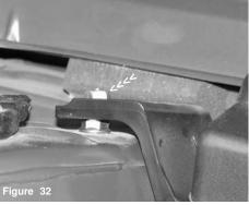
The flange nut is securing the fuse box over the strut tower mount.
