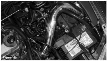
Adjust the entire intake for the best possible fit prior to tightening all nuts, bolts and clamps. Periodically, check the fitment for possible shifting over time. Any shifting may cause damage to moving parts in the engine compartment that may void the warranty.
