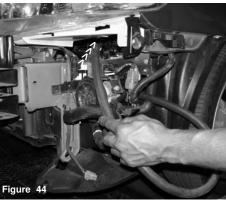
The remaining 15.9mm hose is placed under the head lamp and inserted into the engine compartment.
