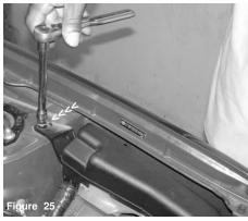
Loosen and remove the m6 nut from the fuse box located on the strut tower mount.
