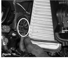
Disconnected the vacuum line at the butterfly valve (VAD) leading from the vacuum switching valve.
