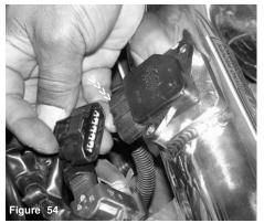
Press the electrical sensor harness into the mass air flow sensor until it snaps firmly in place.
