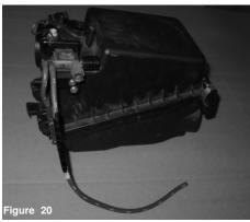
The assembled air box cleaner that has been removed from the engine compartment including the VAD vacuum switching valve,which is no longer used
