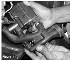
The resonator box and spout is now removed and the spout will be separated from the box as shown above.
