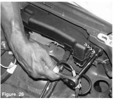
Loosen and remove the m6 bolt on the fuse box located on the fender wall.
