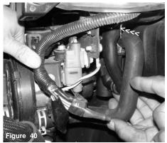
The plastic resonator spout and box are pulled from the upper resonator box with the vacuum hose attached.
