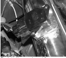
The electrical harness and mass air flow sensor are now completely installed.
