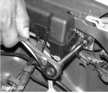
A ratchet and 10mm socket is used to tighten the m6 bolt as shown above.
