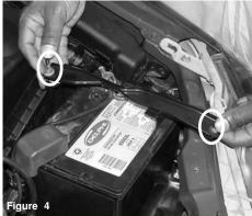
Loosen and remove the two m6 nuts from the battery tie down braces as shown above. Disconnect and remove the battery cables from the battery post.
