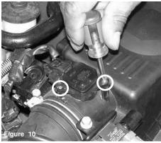
Loosen and remove the two screws located on the mass air flow sensor housing.
