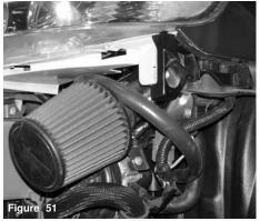
The secondary intake is aligned and in place, make sure that the filter does not hit the bumper when its installed.
