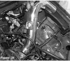
The primary intake is now lowered into the engine compartment. The throttle body end is pressed into the throttle body hose.
