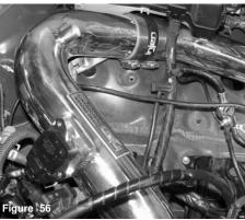
The primary and secondary intakes are now installed and the mass air flow sensor has been inserted into sensor adapter.
