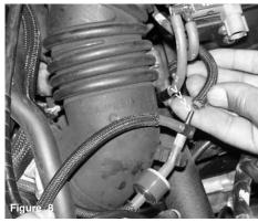
Disconnect the vacuum switching valve line that is connected to the one way check valve.
