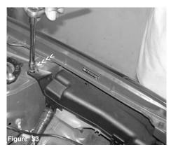
The ratchet and 10mm socket is used to tighten the m6 flange nut over the fuse box.
