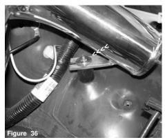
The upper end of the Primary intake is aligned and sitting flush with the vibra-mount stud.
