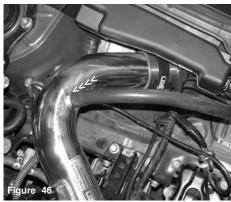
The 15.9mm vacuum line is now connected to the intake vacuum port.
