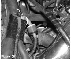
The one way check valve is now secured to the harness.
