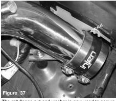
The m6 flange nut and washer is now used to secure the intake in place. The 2 3/4 straight hose is pressed over the primary intake, the power-bands are placed over the hose and tightened.
