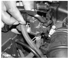
Once you have removed the m6 bolt, continue to pull the VSV from the rubber air duct cradle.
