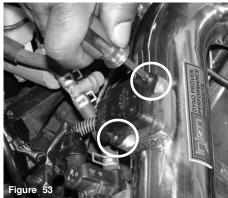
For a better seal, wet the O-ring with light oil prior to inserting the sensor into the sensor adapter. Use the stock screws to secure the sensor to the adapter.
