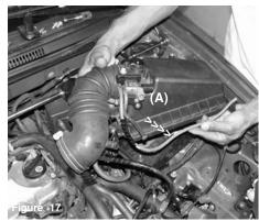
The line that was disconnected from the butterfly valve(VAD) is held to one side (A). The entire top air box cleaner is now removed the the lower air box.
