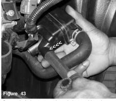
One end of the 15.9mm hose is inserted into the box spout until it is firmly in place.
