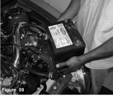
The battery is placed back into the engine compartment and the cables are fastened to the battery post.
