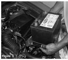
Once the battery tie down has been removed, continue to remove the battery from the battery tray.
