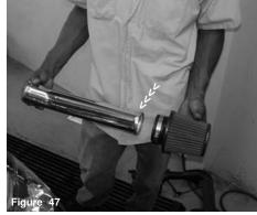
The filter is aligned and pressed over the end of the secondary intake.
