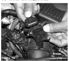
As you remove the mass air flow sensor, unclip the electrical sensor harness as shown above.
