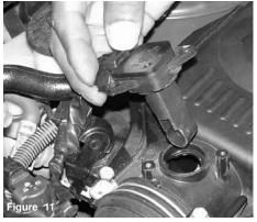
Once you have removed the two screws, continue to remove the mass air flow sensor from the sensor housing.
