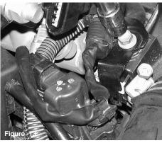
Loosen and remove the PWM vacuum switching valve bolt with a 10 mm socket and ratchet as shown above.
