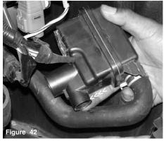
The connecting spout between the lower resonator box and the upper resonator box has been removed from the port shown above.
