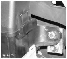
Align the fuse box brace to the upper bracket hole. Use the m6 bolt to secure the fuse box to the bracket.
