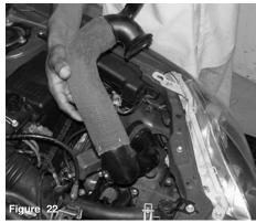
The entire air resonator air duct is now removed from the fender wall as shown above.
