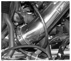
The throttle body end is pressed into the hose and the Power-Band is semi-tightened.
