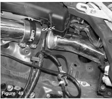
The secondary intake is inserted up into the engine compartment and butted up to the primary intake.
