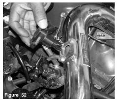
Once the intake has been aligned, continue to insert the mass air flow sensor into the machined sensor adapter.
