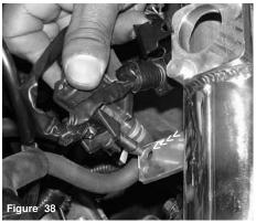
The plastic pin on the PWM vacuum switching valve is inserted into the bracket hole as shown above.
