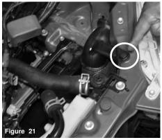
Pull the plastic clip up and remove the clip from the cross member, this will release the air resonator air duct.
