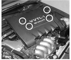
Loosen and remove all four m6 nuts holding the engine cover in place.
