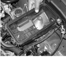
Once you have removed all three bolts, continue to pull the lower air box cleaner from the engine compartment.
