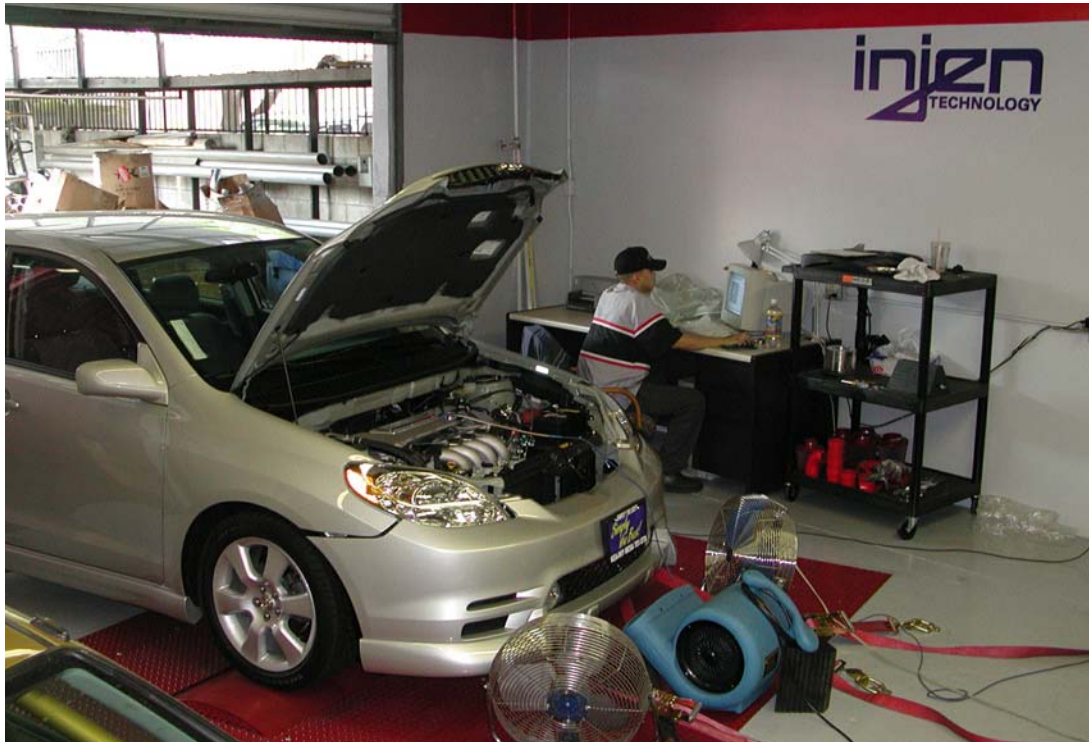
Injen Technology Research & Development Team seen here testing its final design on Injen's own in-ground Dyno-jet. The base horse power run was 157.0 to the wheels. Injen's C.A.I increased its performance to 169.1 h/p that's an increase of 12.1 h/p overall. Torque increase was also seen through-out the band but was noticeable at high end for a total of 7.5 ft./lbs of torque.
