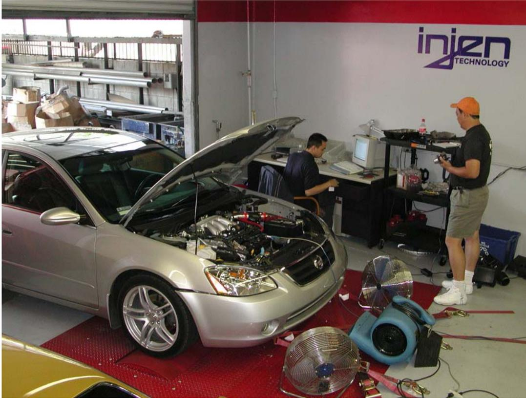
Injen Technology Research & Development Team seen here testing its final design on Injen's in-ground Dyno-jet.
