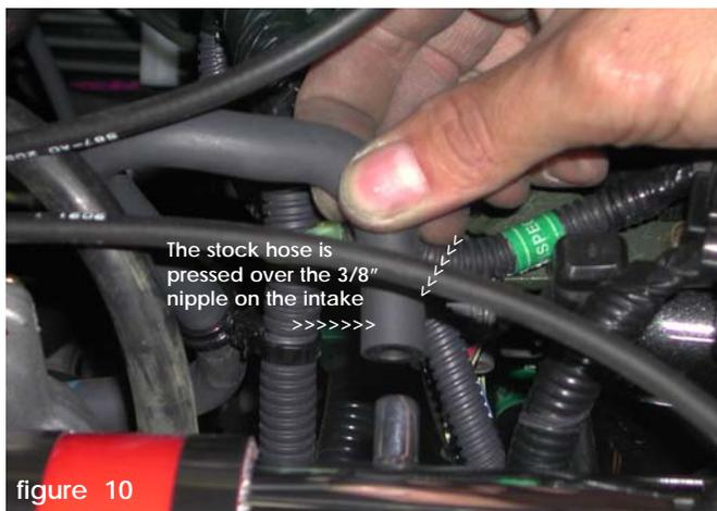
The stock hose is pressed over the 3/8" nipple on the intake >>>>>>
