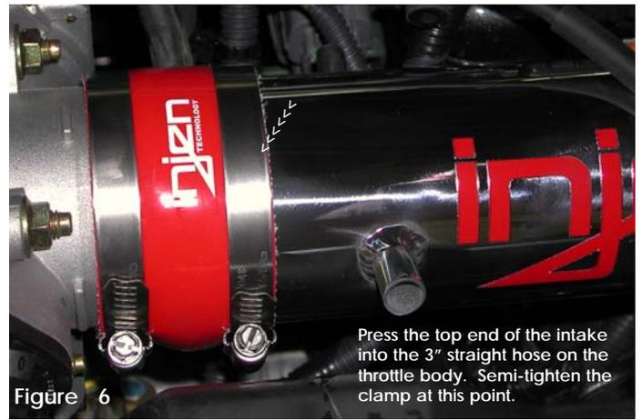
Press the top end of the intake into the 3" straight hose on the throttle body. Semi-tighten the clamp at this point.
