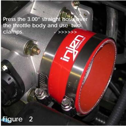
Press the 3.00" straight hose over the throttle body and use two clamps.
