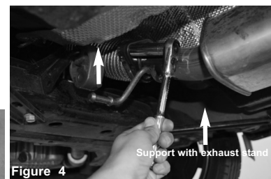
Figure 4 Loosen the 2 15mm nuts on OEM downpipe flange using ratchet and socket. Save nuts and gasket for later use. Remove the factory front section. Support with exhaust stand
