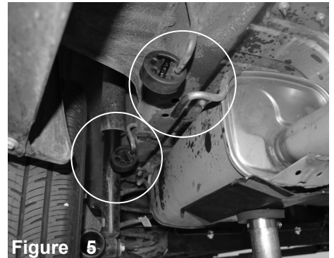
Figure 5 With lubrication, loosen and remove the 3 rubber isolators and remove the rear section of the exhaust.
