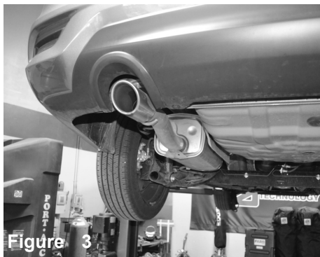
Figure 3 OEM exhaust system. Secure vehicle on lift.
