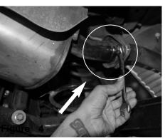
Loosen and remove the rear section of the exhaust using 14m socket or wrench.
