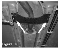
Loosen and remove the frame bracket support using 12mm socket or wrench. This will be re-installed.
