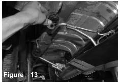
Install rear section using provided M10 nuts and bolts with gasket. Snug fit all bolts and nuts using 14mm socket or wrench. Adjust for clearance and fitment. Make sure tip is centered of exhaust hole cut-out on bumper. Re-adjust if necessary. Use and extra hand for position of muffler and tighten all bolts and nuts. *Exhaust flanges have a alot of room for adjustment.*
