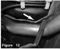
Do to the large pipe diameter, it may come in contact with heat shield, recommended to push back or bend back to have clearance.
