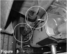
With lubrication, loosen and remove the 3 rubber isolators and remove the rear section of the exhaust.
