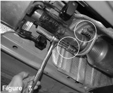
Loosen and remove the front section of the exhaust at the catalytic converter using 14mm socket or wrench.
