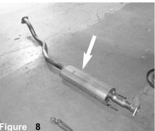
Remove the front section of the exhaust out of the vehicle.
