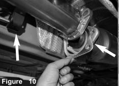
Install the front section of the exhaust. Secure the hangers to the isolators. Secure the flange using provided gasket and 2 M10 bolts. *Do not tighten.*
