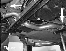
Install the mid section. Install the hangar to the rubber isolation mount. Connect the mid and front section using M10 bolts and nuts with gasket. **Do** not tighten.
