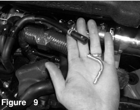
Figure 6 Install the new Turbo auxiliary tube and position to the hose.
