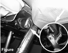
Now install the mid section to the exhaust system, secure the hangar and use provided screws, nuts and gaskets. Do not tighten.
