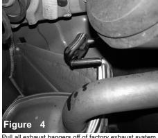
Pull all exhaust hangers off of factory exhaust system, lubricate for easier removal.
