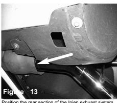
Position the rear section of the Injen exhuast system for enough clearance for the exhaust tip valence.
