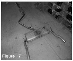
Factory exhaust system fully detached in one piece
