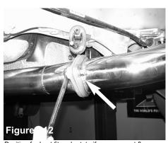
Position for best fit and rotate if necessary at flanges enough for clearance. Tighten all flanges using 9/16" wrench's.
