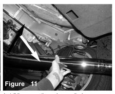
Install the rear section and secure the hangar. Secure the flange with screws provided and gasket. Do not tighten.
