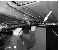
Install the front section of the exhaust and secure the hangars to the rubber isolators.
