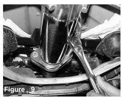
Secure the flange using factory nuts. Tighten using 12mm deep socket.
