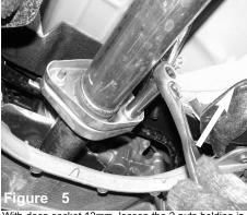
With deep socket 12mm, loosen the 2 nuts holding in the exhaust flange at the CAT. Save screws for later install.
