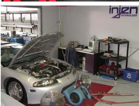
Injen Research and Development Team testing various proto-types on the dyno-jet. Both short intakes and cold air intakes are tested repeatedly.
