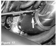
Once you have adjusted the intake and 45 degree elbow for the best possible fitment, tighten the two clamps on the 45 degree elbow
