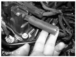
Attach the provided 12mm hose to the crank case fitting on engine.
