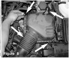
unlatch to remove the upper portion of the factory air box cleaner
