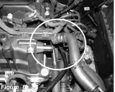
Remove the crank case line from the vehicle. If equipped with the brake booster line, disconnect from the intake and save for later install.
