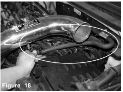
(MANUAL TRANSMISSION ONLY) Place the vacuum line from the brake booster to the 3/8" straight nipple underneath the intake pipe. Make sure to reuse the pressure clamps to secure the vacuum line.
