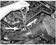
Use a plier and loosen the two pressure clamps on the two breather lines on the air box air duct.
