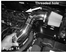
Install the intake system. Line up the intake bracket next to the threaded insert on the valve cover.
