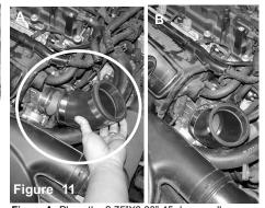
Figure A: Place the 2.75"X3.00" 45 degree elbow with two 48 clamps onto the throttle body . Make sure the 2.75" side goes oonto the throttle body. Figure B: Hose shown on throttle body
