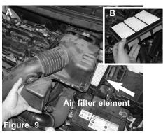
Figure A: Remove the entire upper portion of the air box cleaner. Figure B: Now remove the air cleaner element. This filter will no longer be used in this installation
