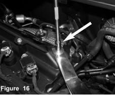
Locate the insert on the valve cover, and secure the bracket using provided M6 screw and fender washer. Tighten using 10mm socket and ratchet.
