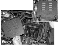
Figure A: Place the Injen AIr box ventilation cover onto the top of the air box cleaner and use factory latch to keep cover in place. Figure B: Injen Cover shown on top of factory air box
