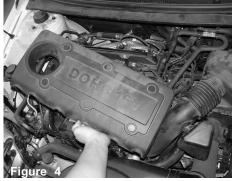
Remove the plastic engine cover by firmly lifting up.
