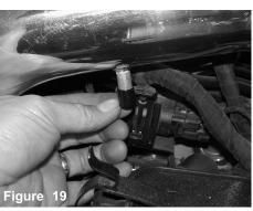
(AUTOMATIC MODELS ONLY) Place the 8mm cap onto the 3/8" nipple
