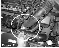
Use a 10mm socket and rachet to loosen the clamp on There are four retaining clips that you will have to the air duct connected to the throttle body
