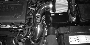
Congratulations! You have just completed the installation of this intake system. Periodically, check the alignment of the intake, normal wear and tear can cause nuts and bolts to come loose. Failure to check the alignment and adjust the intake can cause damage that will void the warranty.
