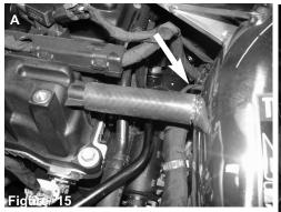
Secure the crank case line to the fitting on the intake tube.
