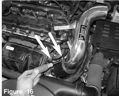
Figure 16 Once you have adjusted the intake and 45 degree elbow for the best possible fitment, tighten the two clamps on the 45 degree elbow
