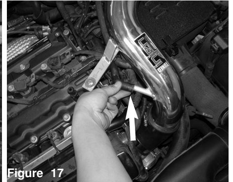
Figure 17 Place the breather port on the valve cover onto the 1/2" angled nipple welded to the intake pipe. make sure to place the pressure clamp back onto the breather line
