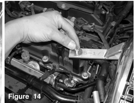
Figure 14 Place the M6X25 bolt and fender washer to secure the intake to the threaded hole on the valve cover
