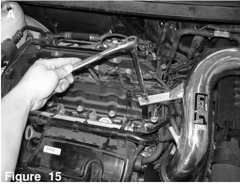
Figure 15 Use a 10mm socket and ratchet to secure intake bracket onto the engine valve cover.
