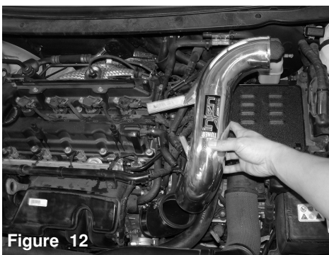
Figure 12 Place the intake tube into the 45 degree elbow
