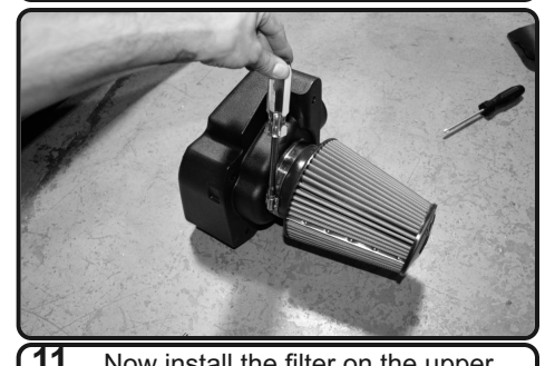
11. Now install the filter on the upper plenum air box. Secure and tighten using 8mm nut driver.
