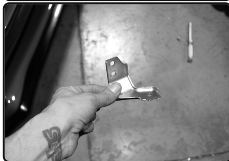
9. Remove the factory bracket from the OEM air box.
