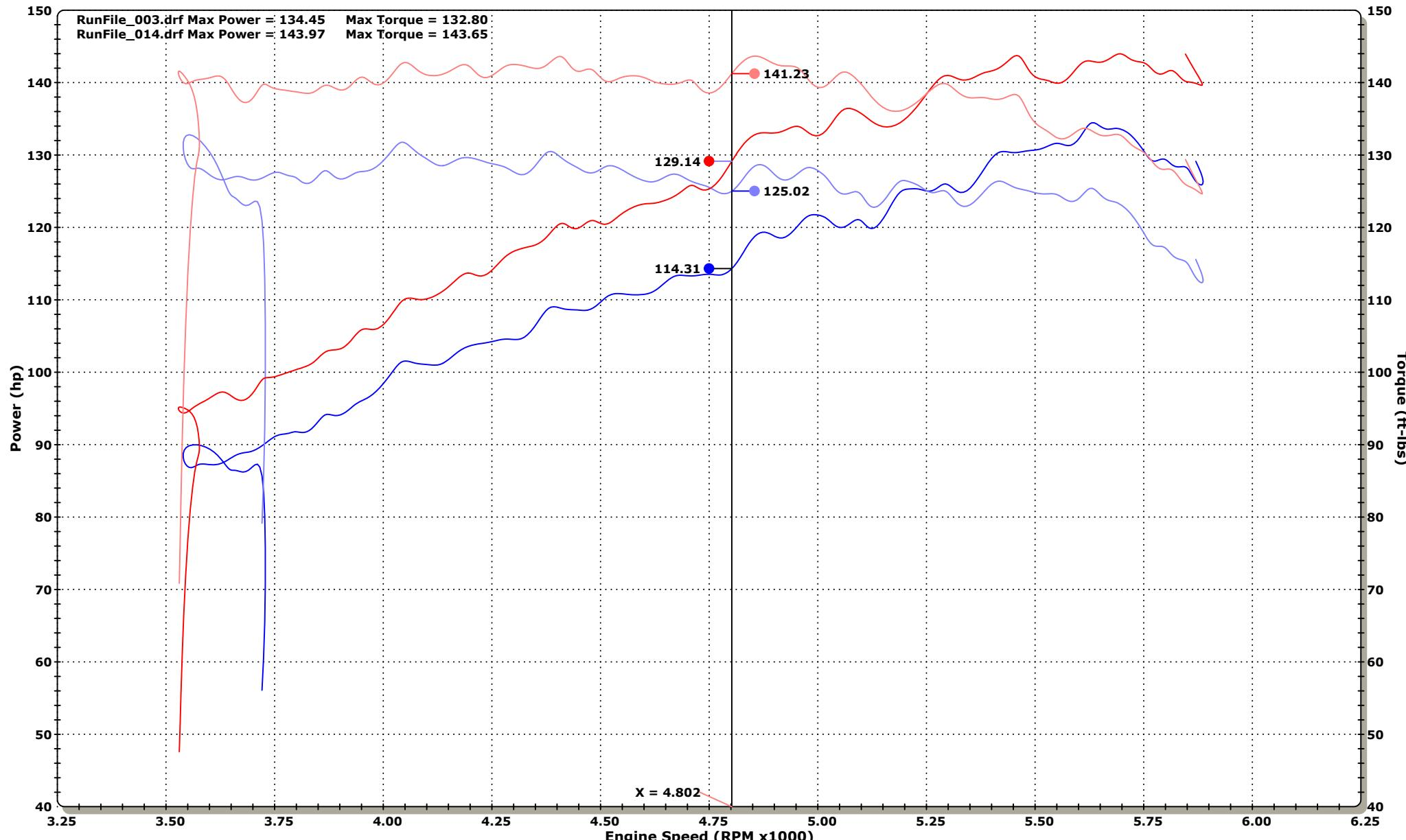
RunFile\_003.drf - 3/3/2011 10:41:12 AM Run Type: RO Run Conditions: 69.25 °F, 29.36 in-Hg, Humidity: 42%, SAE: 1.00
