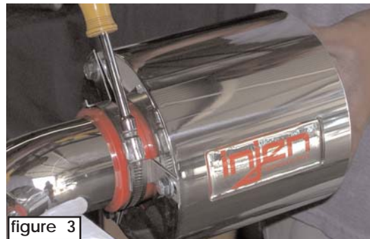
figure 3 Once the filter is aligned continue to tighten the clamp over the intake.
