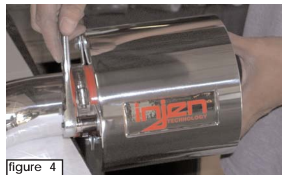
figure 4 Check all 5/16" flange bolts for proper fit and adjustment.
